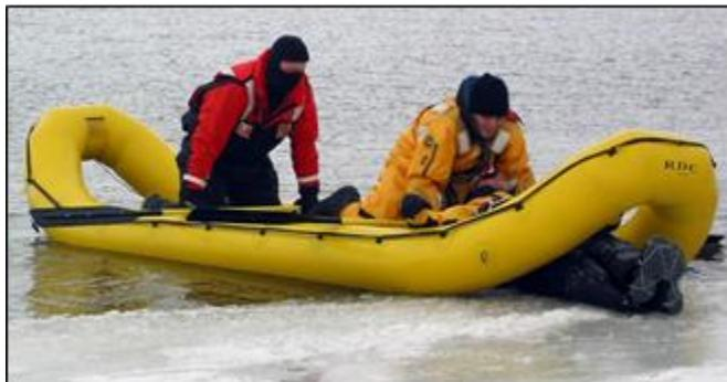
**MARSARS rescue sled** – a sled that can propelled across the ice to a victim. As the sled nears a victim the empty sled becomes a self-rescue reaching device for victims that can assist in own rescue. The sled provides for a quicker extraction by minimizing risk of injury to both victim and rescuer.
