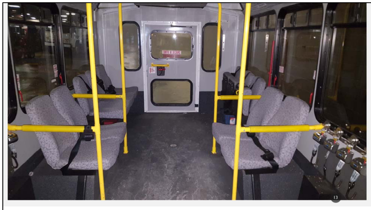
Inside the ARBOC bus looking towards the back. The very back seats can flip up to expose two wheelchair spots.
