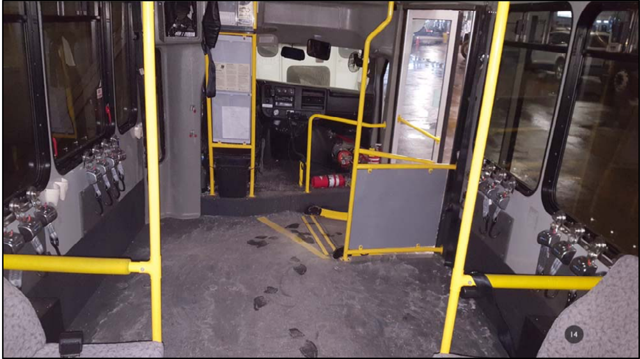
Inside the ARBOC bus standing at the back looking forward. Note the space for wheelchairs and the greater width of the floor space relative to the Promaster.
