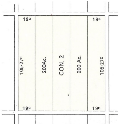
Figure 2: The single front survey system, used from 1783 to 1818. As depicted here, each lot is 200 acres (Ac.), created from surveying 19 chains by 105.27 chains (1 chain = 66 feet/ 20.12 metres) (Gentilcore 1969:61)
