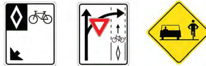
Exhibit 41 - Examples of signage for on-road cycling facilities (TAC RB-19, TAC RB-37, OTM Wc-19)
