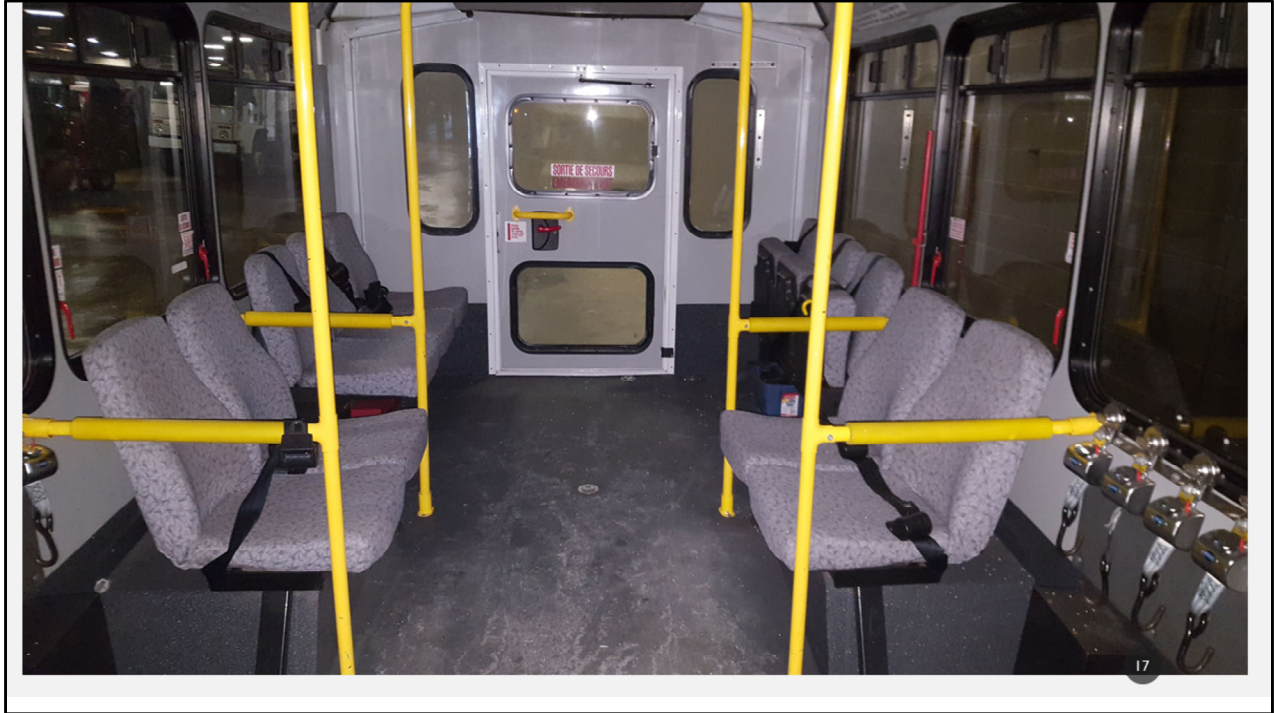
Inside the ARBOC bus looking towards the back. The very back seats can flip up to expose two wheelchair spots.
