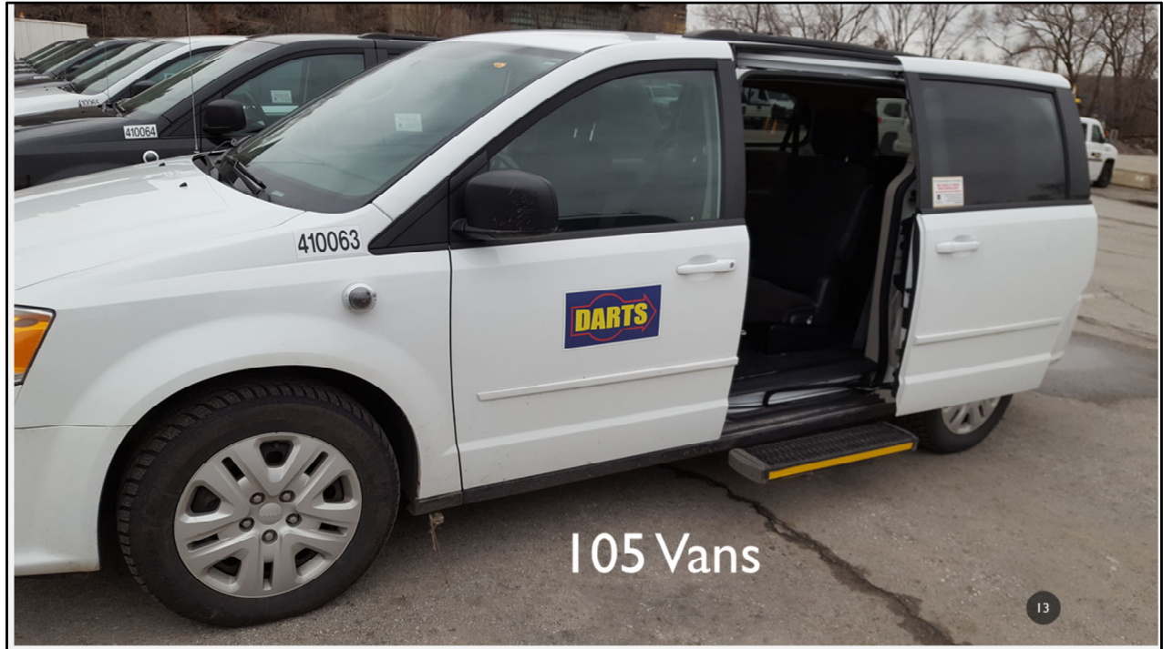
DARTS van showing the installed step (these are on both sides of the vehicle) to assist seniors with entering the van.
