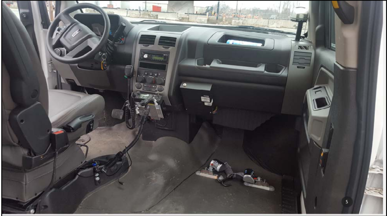
Inside the MV-1 vehicle looking forward. Shows the position of the one wheelchair spot in the front passenger position.
