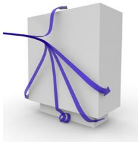
b) Downwashing Wind Flow Around Buildings with Podiums (Left) and Undercuts (Right)
