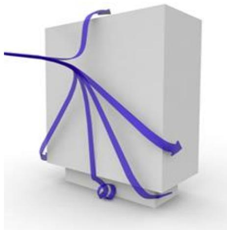
b) Downwashing Wind Flow Around Buildings with Podiums (Left) and Undercuts (Right)
