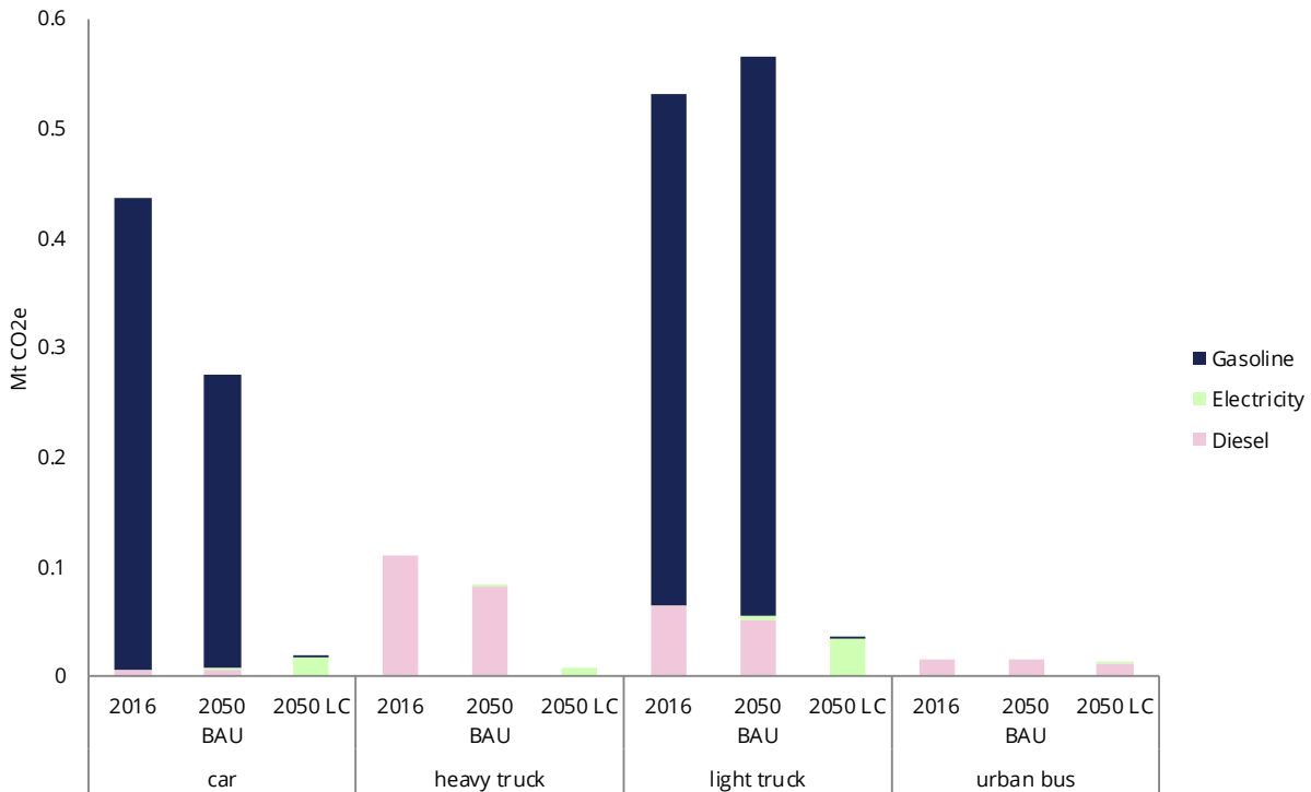
Figure 68. Projected transportation GHG emissions (MtCO 2 e) by source and vehicle type, Hamilton.
