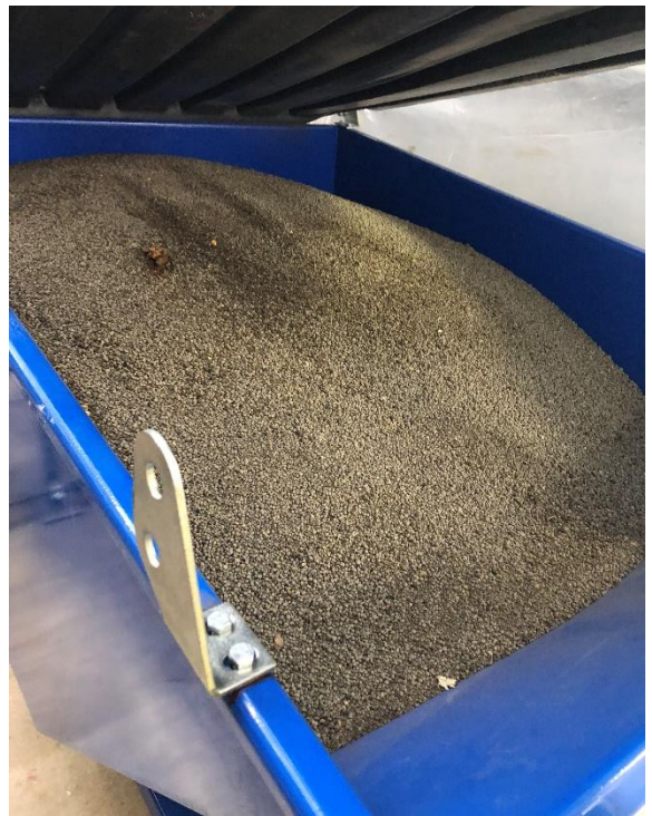
Figure 10: Final Product, Dry Pellets
