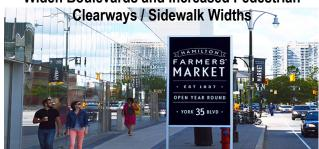
Widening boulevards and sidewalks may be appropriate in areas with high volumes of pedestrian traffic. Wider unobstructed pedestrian pathways (clearway) provides the space necessary for pedestrians to pass, push strollers, or navigate using mobility assistive devices.
