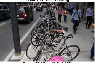
Bike parking describes any end-of-trip facility that is designated for locking bicycles. Bike racks are a common form of bike parking typically placed in the boulevard. These facilities are used for short-term parking and should be located where pedestrian traffic is high to deter vandalism and theft through passive surveillance.
