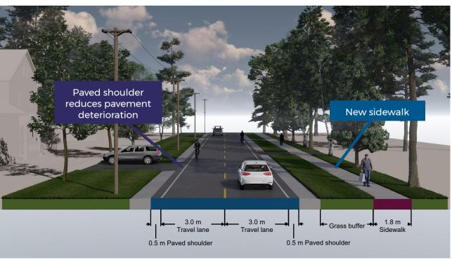
Rural Settlement Roads are portions of Rural Roads that pass through village, and may include residential frontages or commercial uses. In this example, traffic volumes and speeds are relatively low, and a small paved shoulder is provided to improve pavement longevity and reduce maintenance costs.
