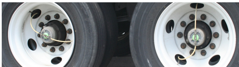
Figure 24: Automatic Tire Inflation System (courtesy NACFE)
