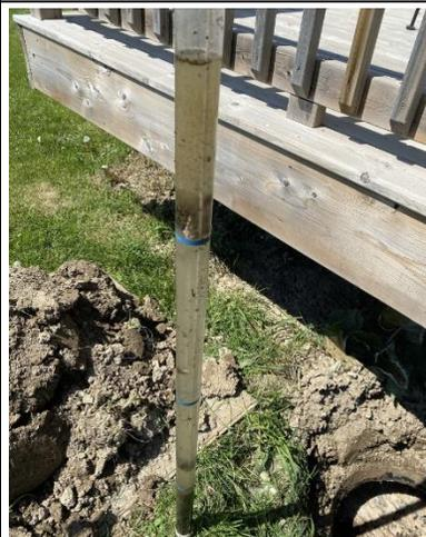
6. Sludge measurement of system (1 compartment) 35% solids – requires pump-out
