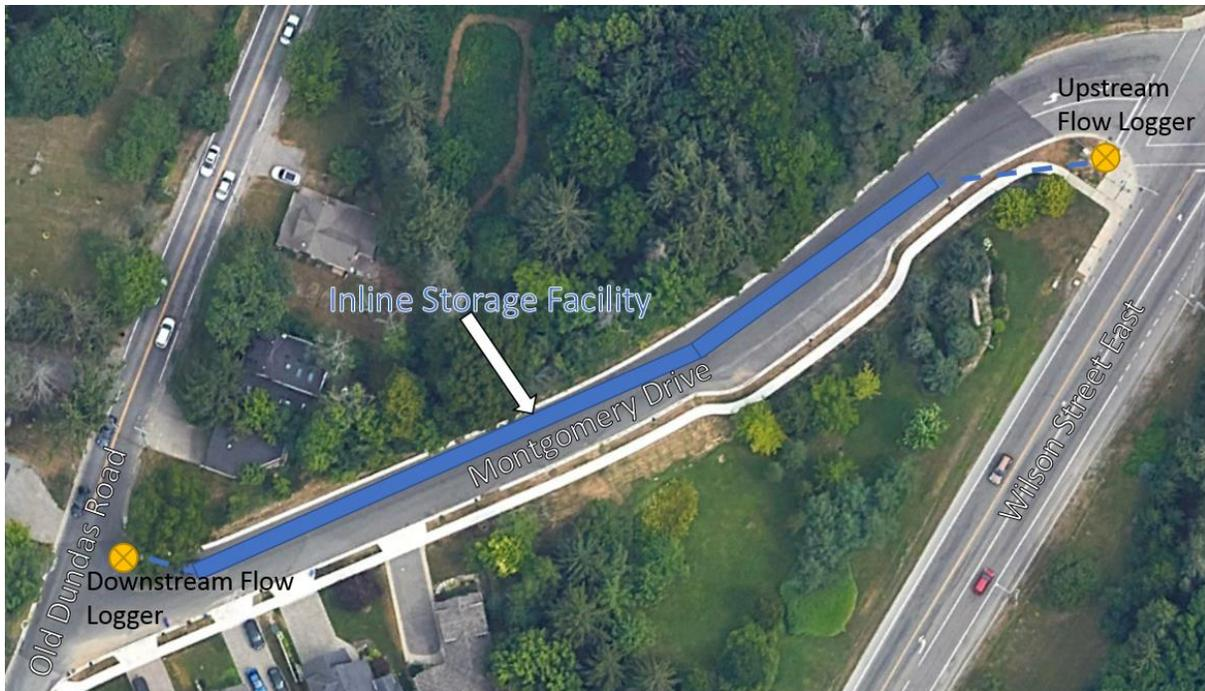
**Figure 1.5: Locations of Sanitary Flow Loggers**
