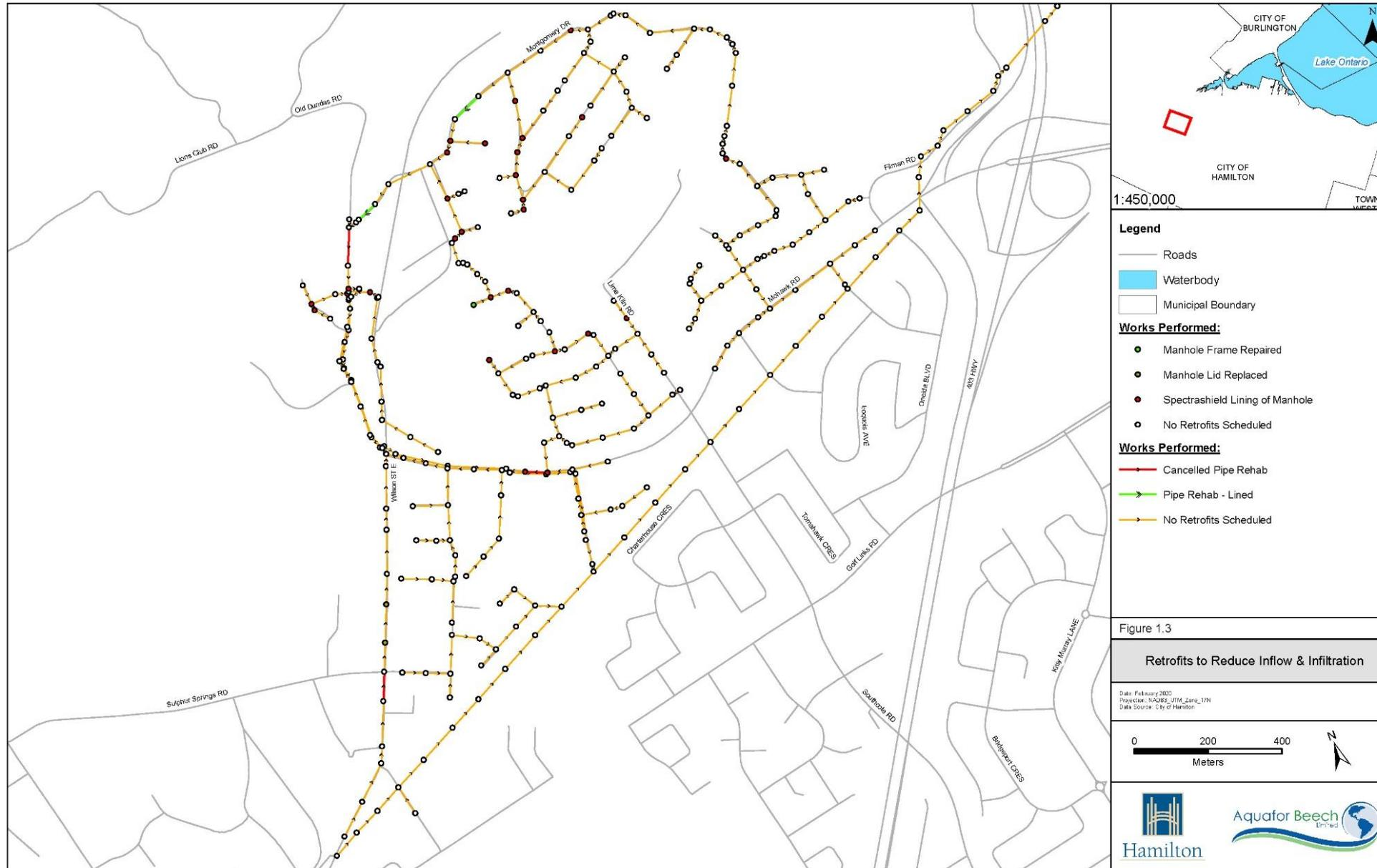
Figure 1.3: Retrofits to Reduce Infiltration / Inflow
