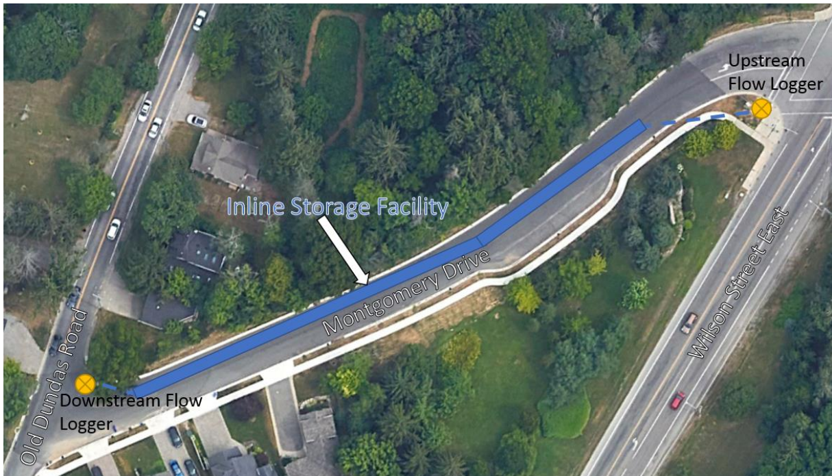
Figure 1.5: Locations of Sanitary Flow Loggers
