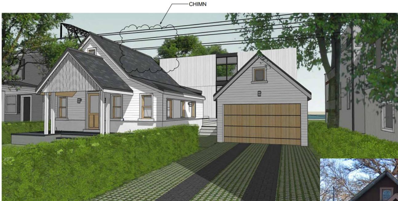
**Proposed Elevation** – only change visually is removal of chimney and some window openings in order to meet current OBC code
