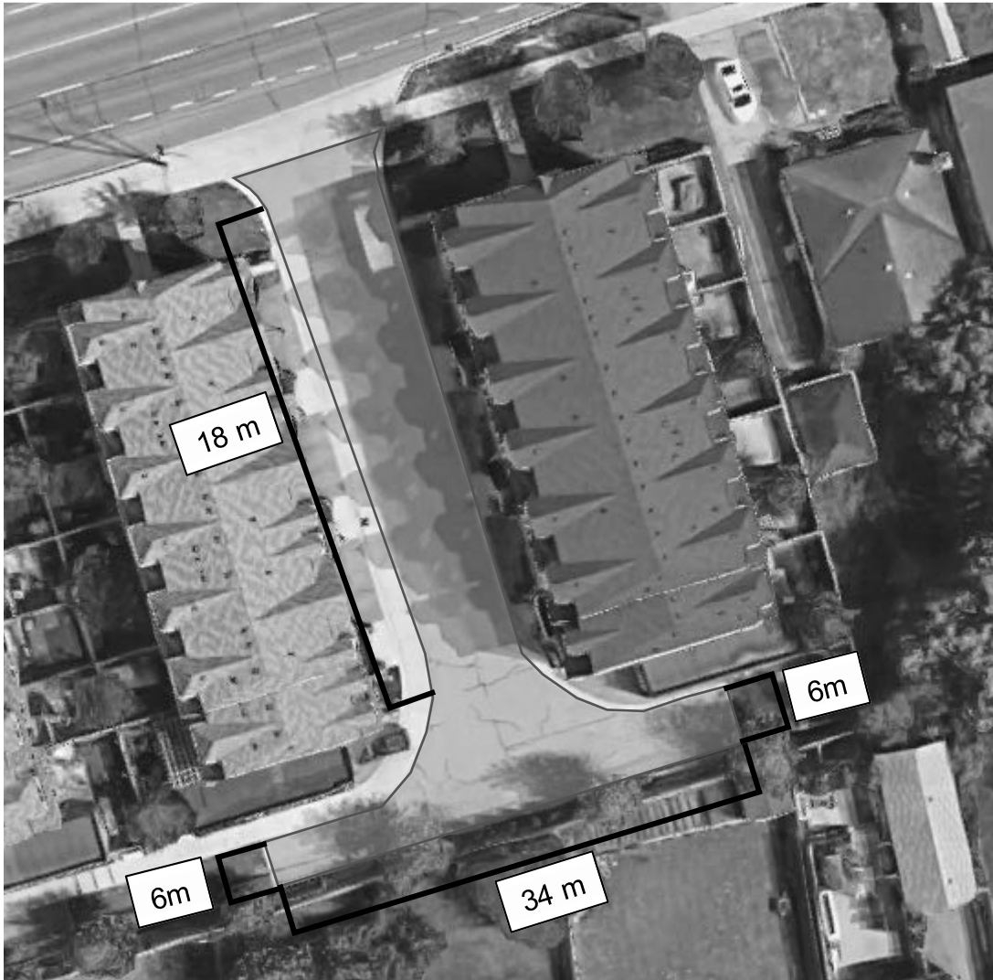
Figure 2: Satellite image showing a T-Turn in a subdivision which would be acceptable to Waste Collections. Diagram is not to scale.
