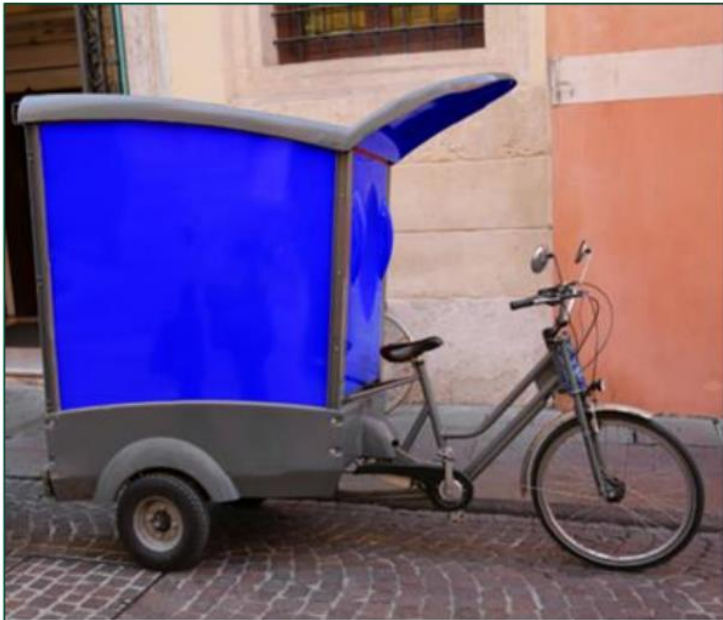
Tricycle cargo e-bike design with enclosed cargo box at the back
