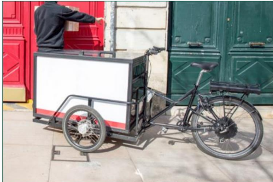
Reverse tricycle design with enclosed cargo box in the front
