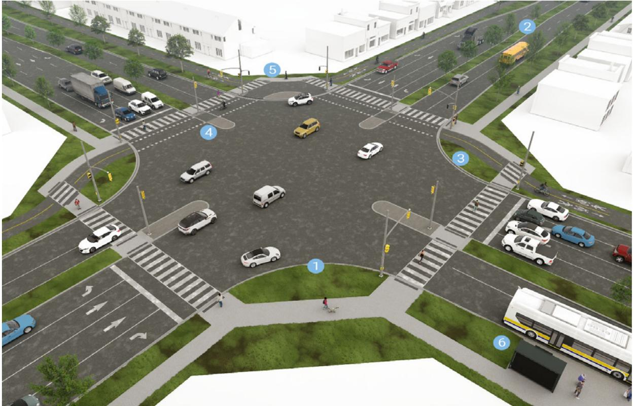
This intersection is an example of two high-capacity Transitioning Avenues intersecting. Due to the high volumes of turning vehicles expected at these intersections, the intersection is designed with the intention that protected signal phasing will be used to minimize conflicts between turning vehicles and pedestrians or cyclists.
