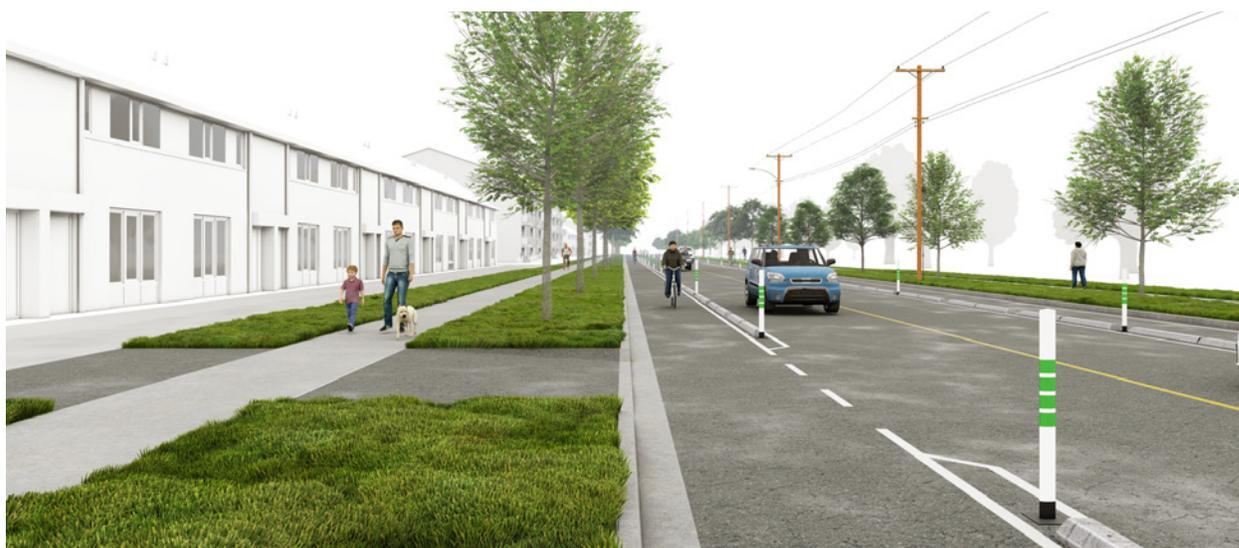
*Cross-section of one-way physically separated bike lanes.*
