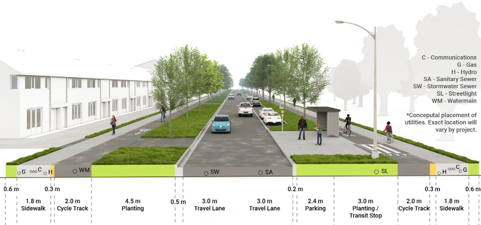
Typical Connector Cross Section (26m ROW)–New Construction.
