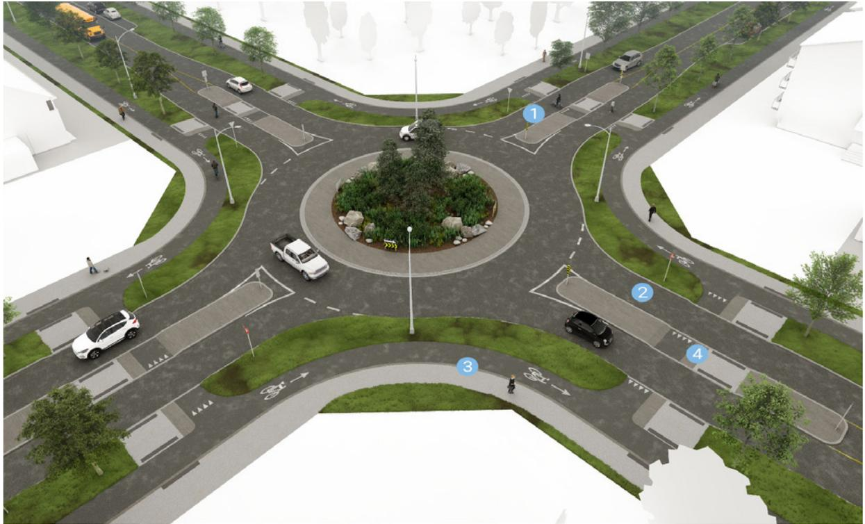
This example of a roundabout intersection between two Connector Streets draws on design guidance from OTM Book 18: Cycling Facilities, the TAC Canadian Roundabout Design Guide, and NCHRP Report 672, Roundabouts: An Informational Guide . Roundabouts typically require more right of way space than traditional intersections, as such property requirement needs should be an early consideration in the roundabout design process.
