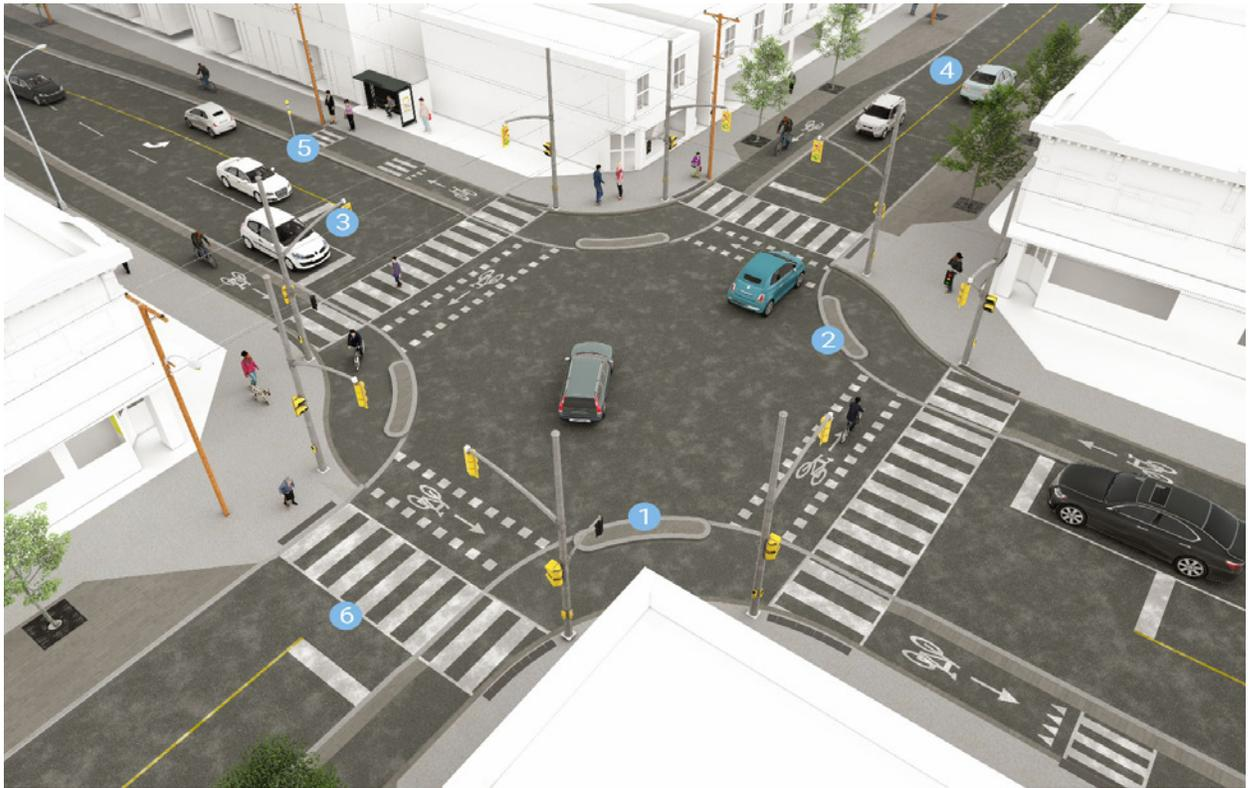
This intersection is an example of a signalized compact urban intersection. The design of this intersection aims to separate and protect vulnerable road users as much as possible to minimize conflicts with motor vehicles. The design shows an intersection of an Urban Avenue and a Main Street. For intersections of two Urban Avenues, the design of the Urban Avenue approaches can be replicated on all four legs of the intersection.
