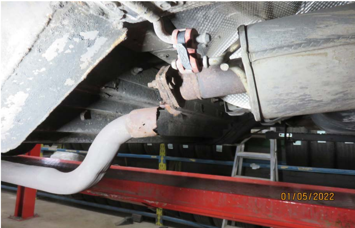
- 98 Figure 11. DARTS #410106 Exhaust broken off. Image by FCC Inc.
