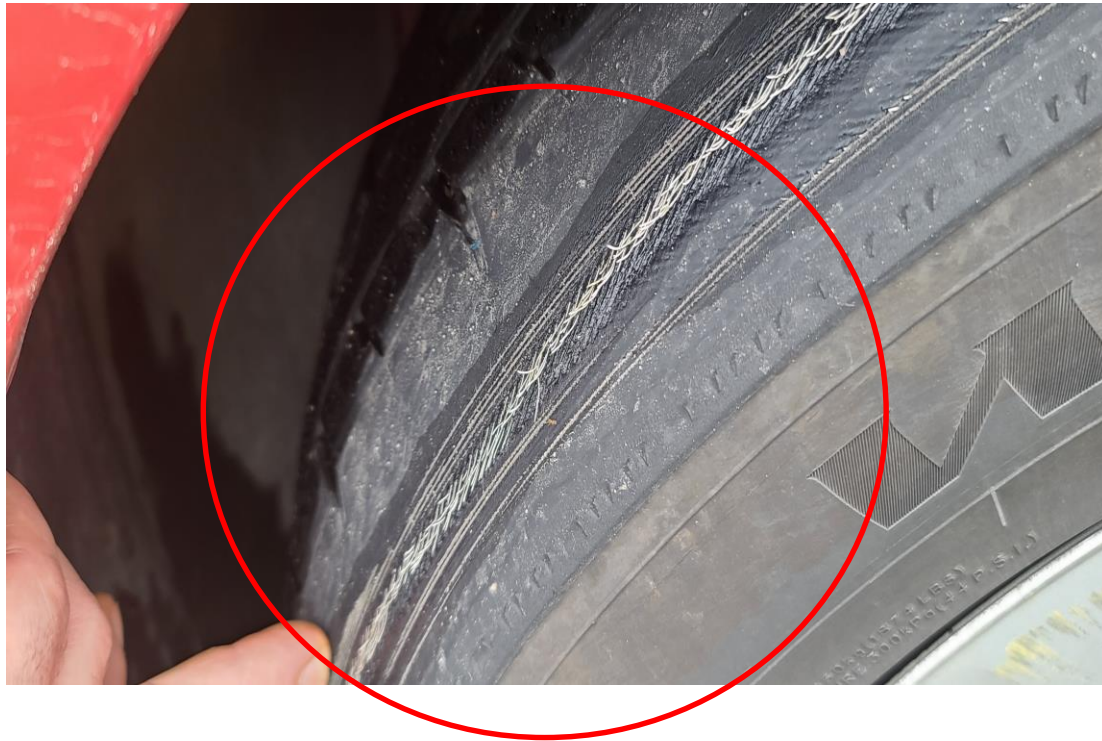
Figure 8. Vankleef #606 bald tire with steel cords exposed. Image by OCA
