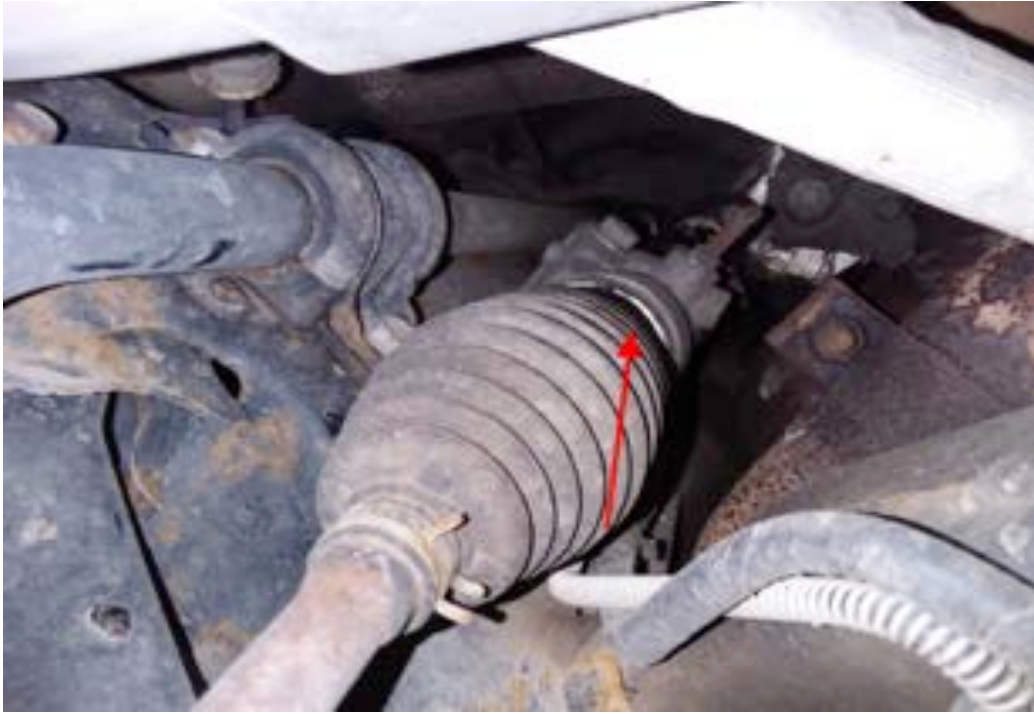
Figure 6. Vankleef #611. Both inner tie rod boots torn. Image by AG&R
