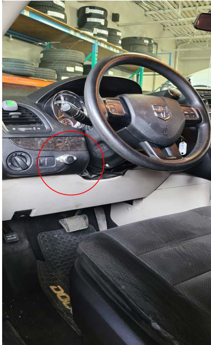
Figure 10. City Marvel #CV218 – Auxiliary horn button unlabelled, not OEM. Factory horn non-functional. Image by OCA
