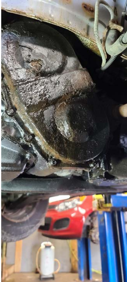
Figure 1. H-Rising #HV113 major oil leak - Image by OCA
