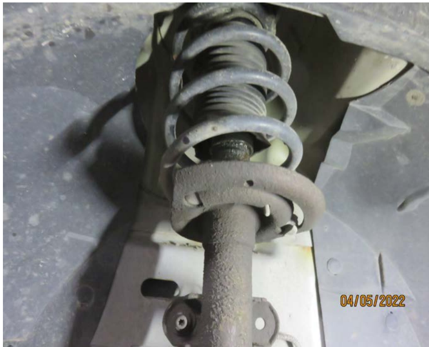
Figure 9. City Marvel #CV203 - Strut leaking. Image by FCC Inc.
