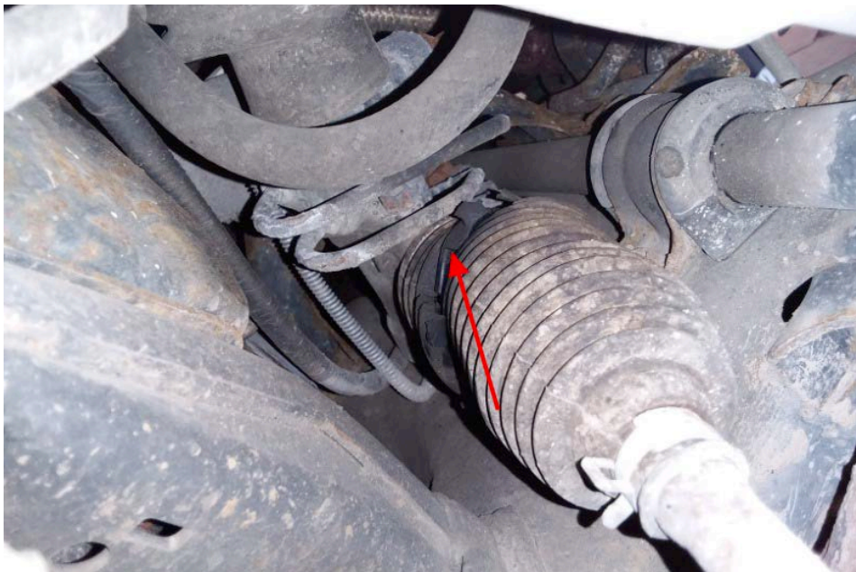
Figure 7. Vankleef #672 Split inner tie rod boot. Image by AG&R
