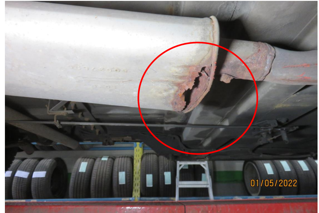
Figure 12. DARTS Unit #410107 - Large hole rusted in muffler. Image by FCC Inc.
