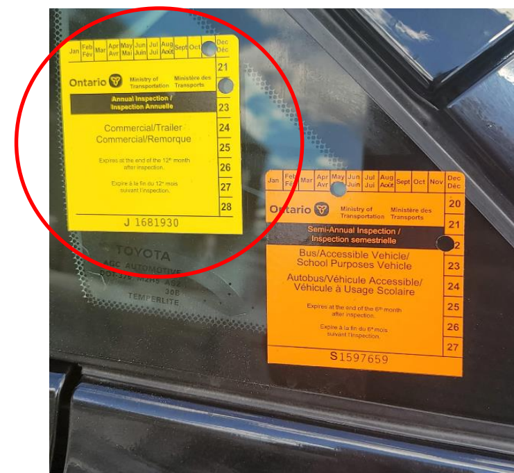
Figure 2. H-Rising #HS102 Incorrect safety (trailer) inspection sticker installed. Shown with correct sticker applied later. Image by OCA
