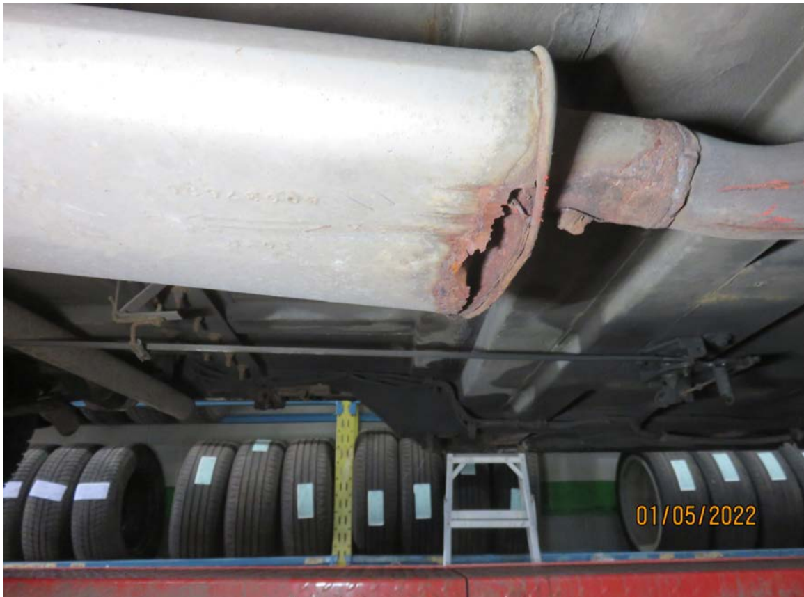
Figure 12. DARTS Unit #410107 - Large hole rusted in muffler. Image by FCC Inc.
