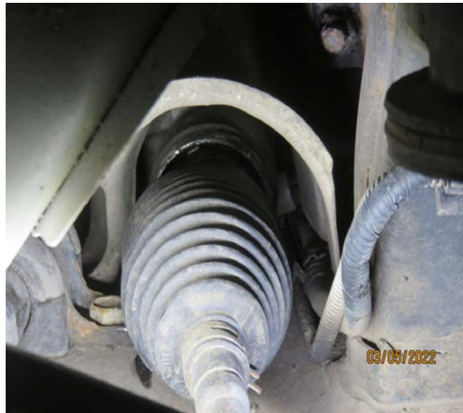
Figure 3. H-Rising #HV103 CV Joint boot broken/split. Image by FCC Inc.
