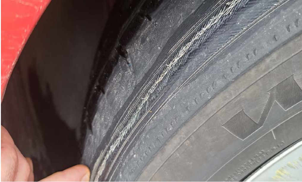
Figure 8. Vankleef #606 bald tire with steel cords exposed. Image by OCA
