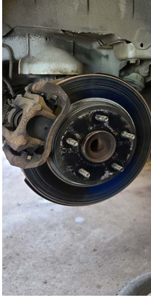
Figure 13. City Marvel #CV211. Seized brake caliper. Image by OCA.
