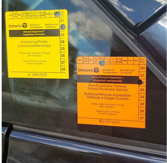
Figure 2. H-Rising #HS102 Incorrect safety (trailer) inspection sticker installed. Shown with correct sticker applied later. Image by OCA
