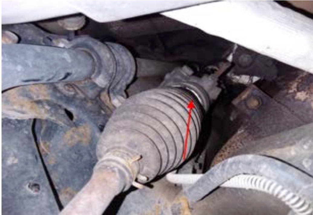
Figure 6. Vankleef #611. Both inner tie rod boots torn. Image by AG&R
