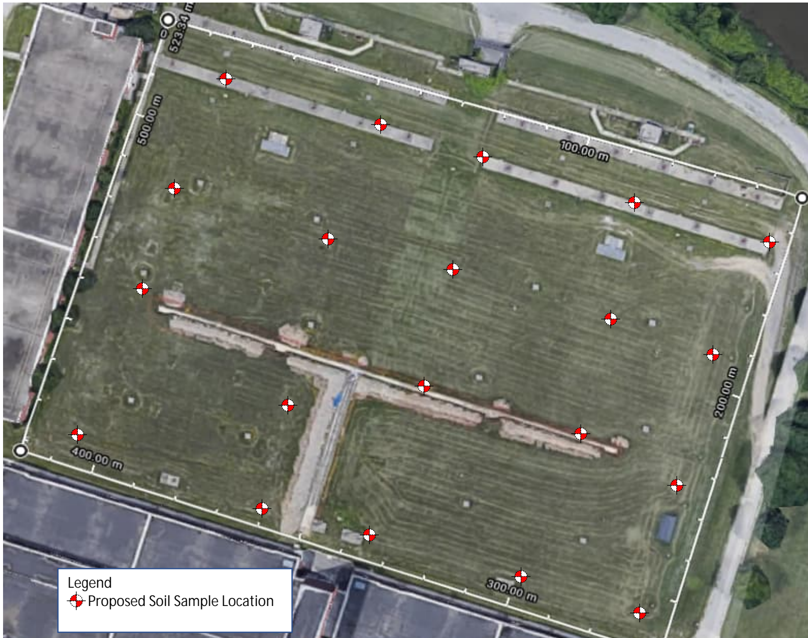
Figure 13: Sampling Locations for Woodward Ave. Water Treatment Plant - Sedimentation Tanks
