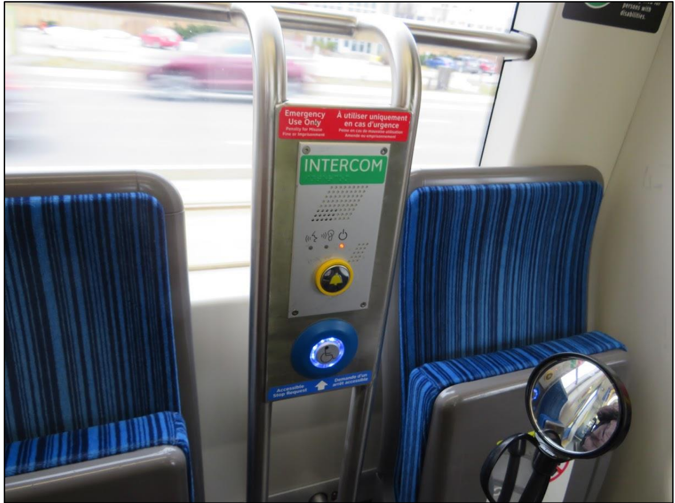
Figure 24: Emergency Intercom on the LRV as well as the Accessible call button to alert the operator that more time is needed to disembark. Connects camera so operator can ensure no issues
