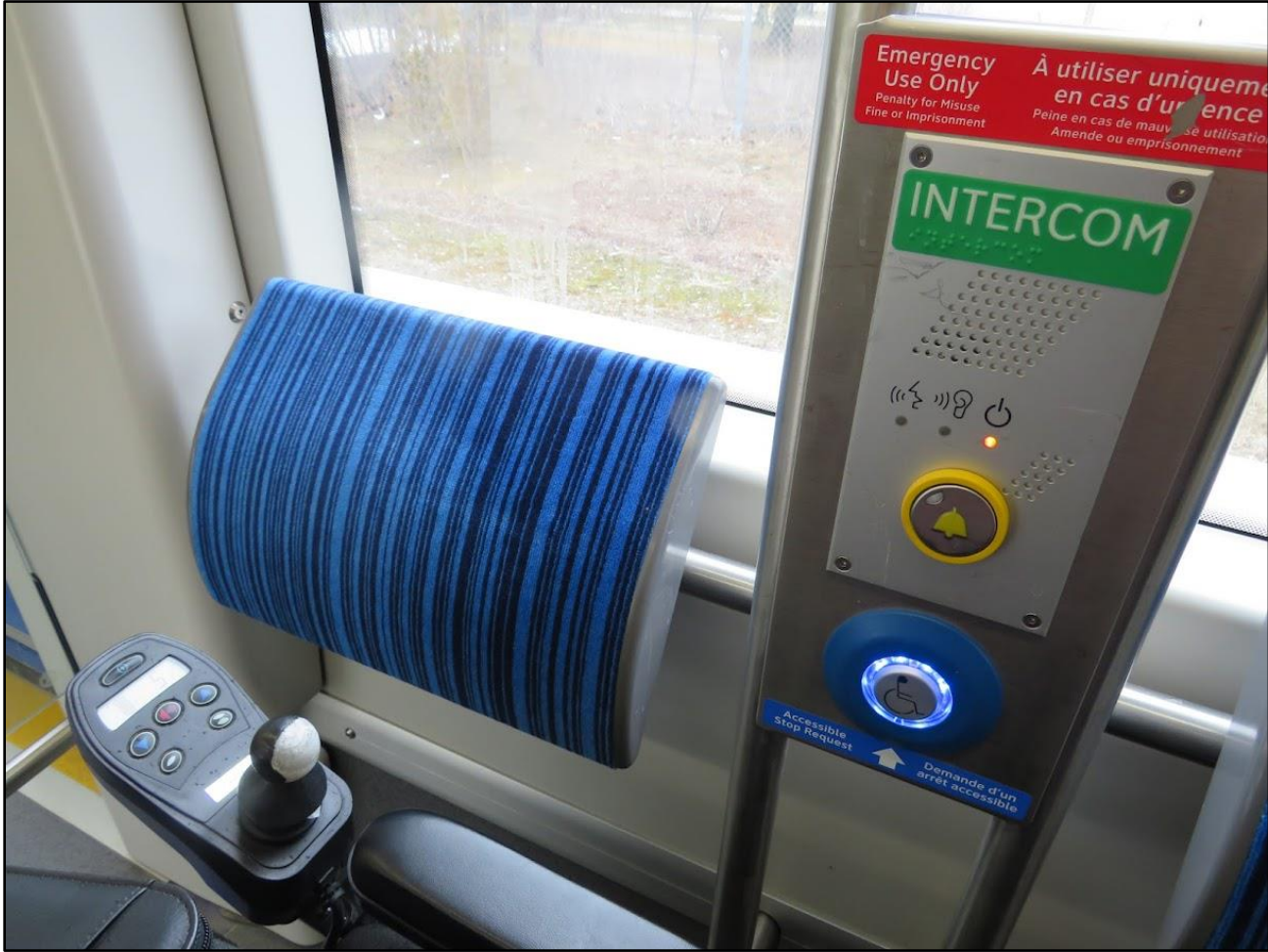
Figure 44: Emergency intercom, call button and lean against seating. *Each train has a set of foldable seats and half benches you lean against.
