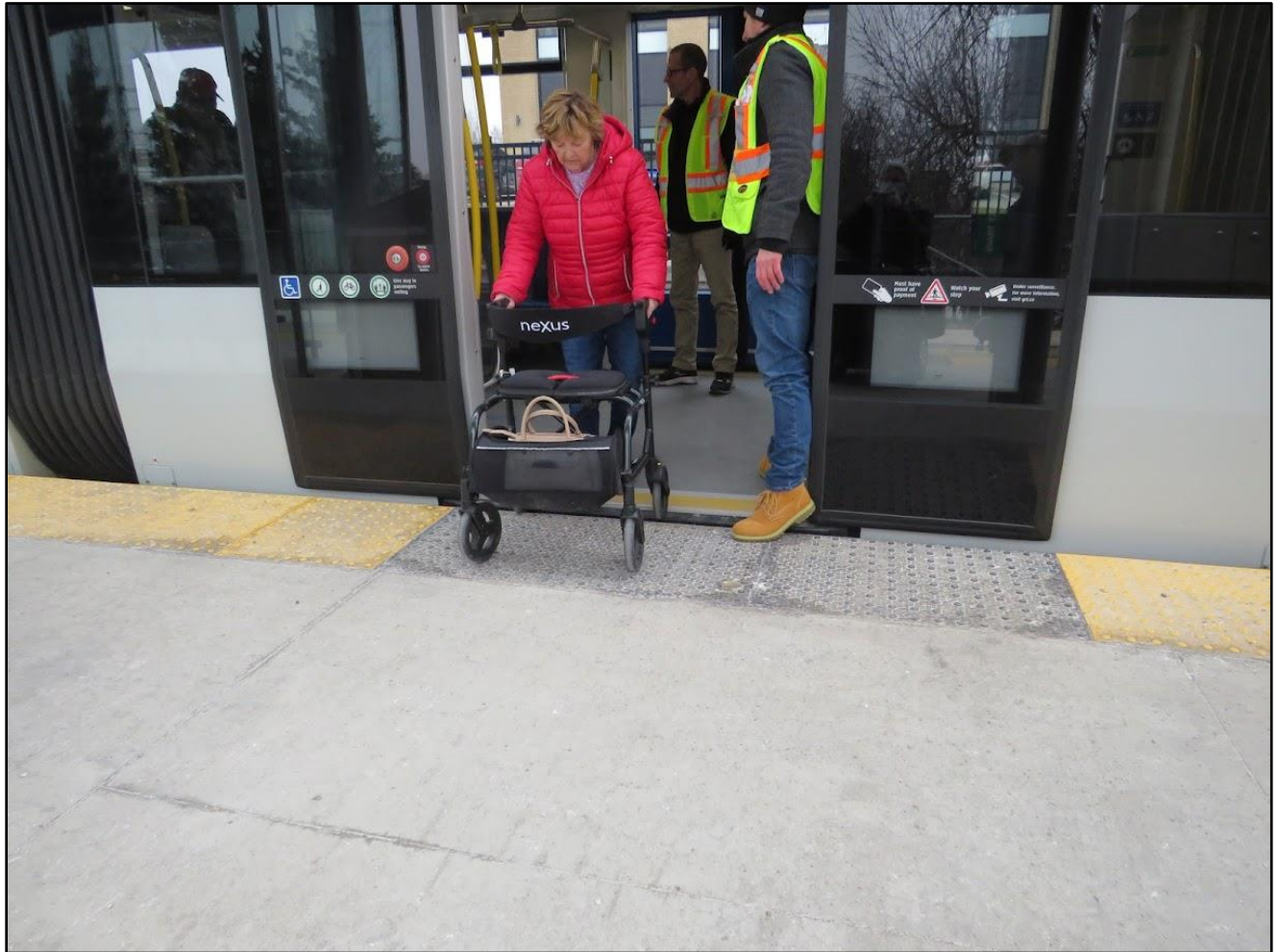
Figure 23: Disembarking from the train. *The step off is significant for little wheels.
