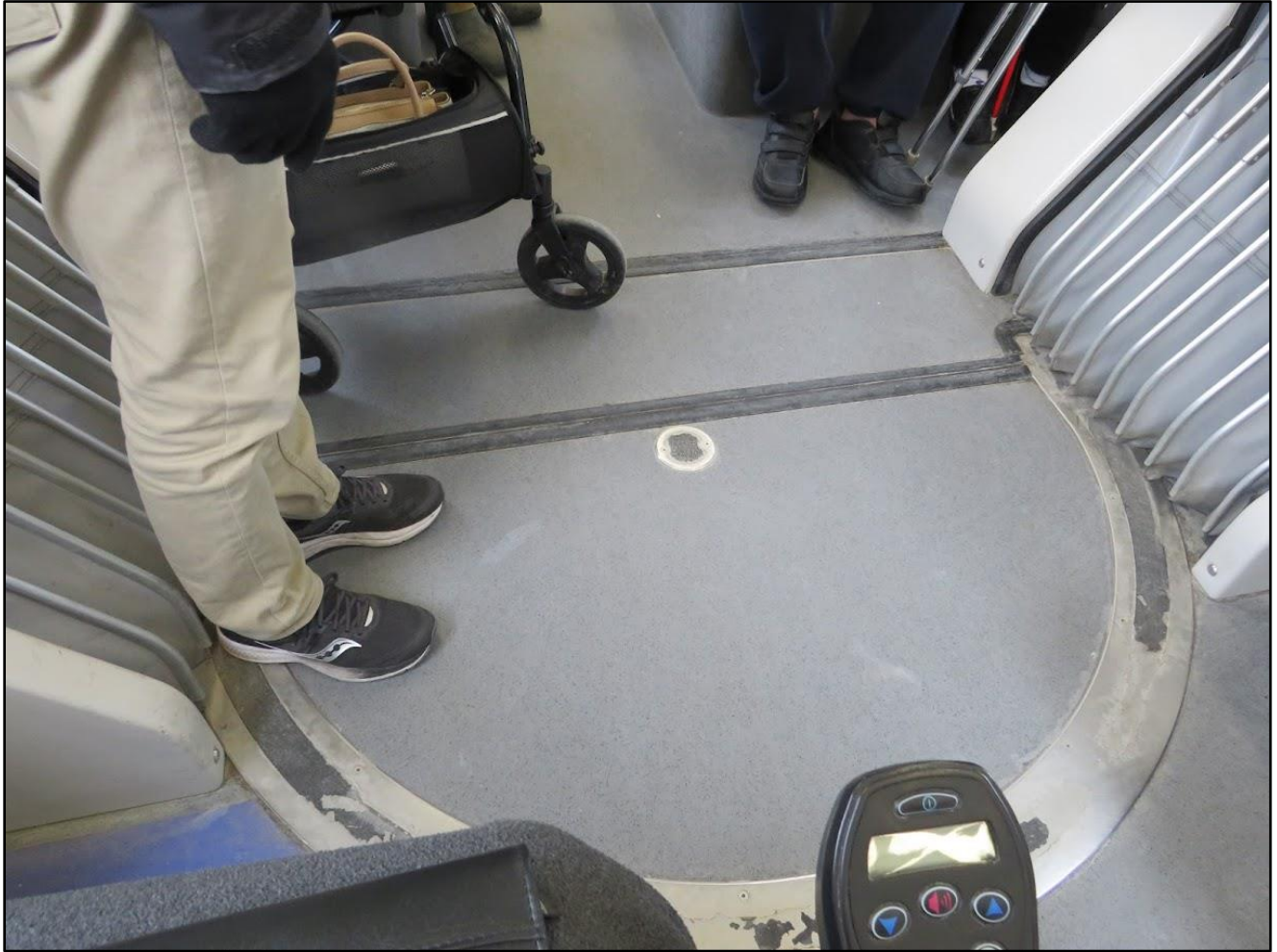
Figure 26: Design of LRV vehicle and where the floor shifts to align with the track (similar to an articulated bus) *This is a problem area for mobility devices. You have to make certain you are not on the metal area or it will shift the device.
