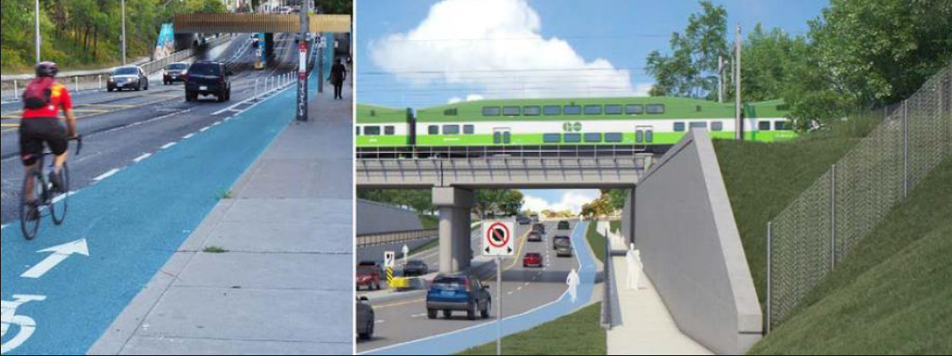
EXAMPLE: GO EXPANSION PROJECTS Accommodating planned municipal bike lanes as part of a grade separation project.
