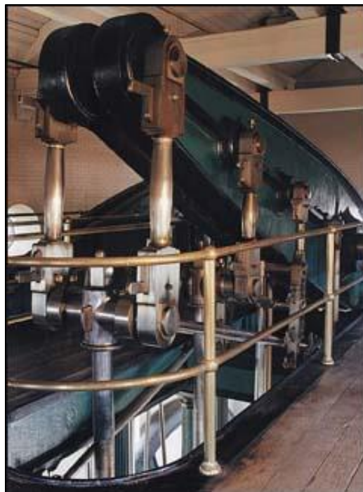
Figure 5: Walking beam of one of the steam engines produced for the Hamilton Water Works in 1859 by the Dundas Foundry following its restoration in 1998 (Source: https://esemag.com/archives/november-1998-hamiltons-historic-waterworks-steam-engines-now-restoredto-mint-condition/ )
