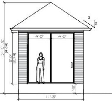
2 NORTH POOL HOUSE ELEVATION SCALE: 1/16" = 1'
