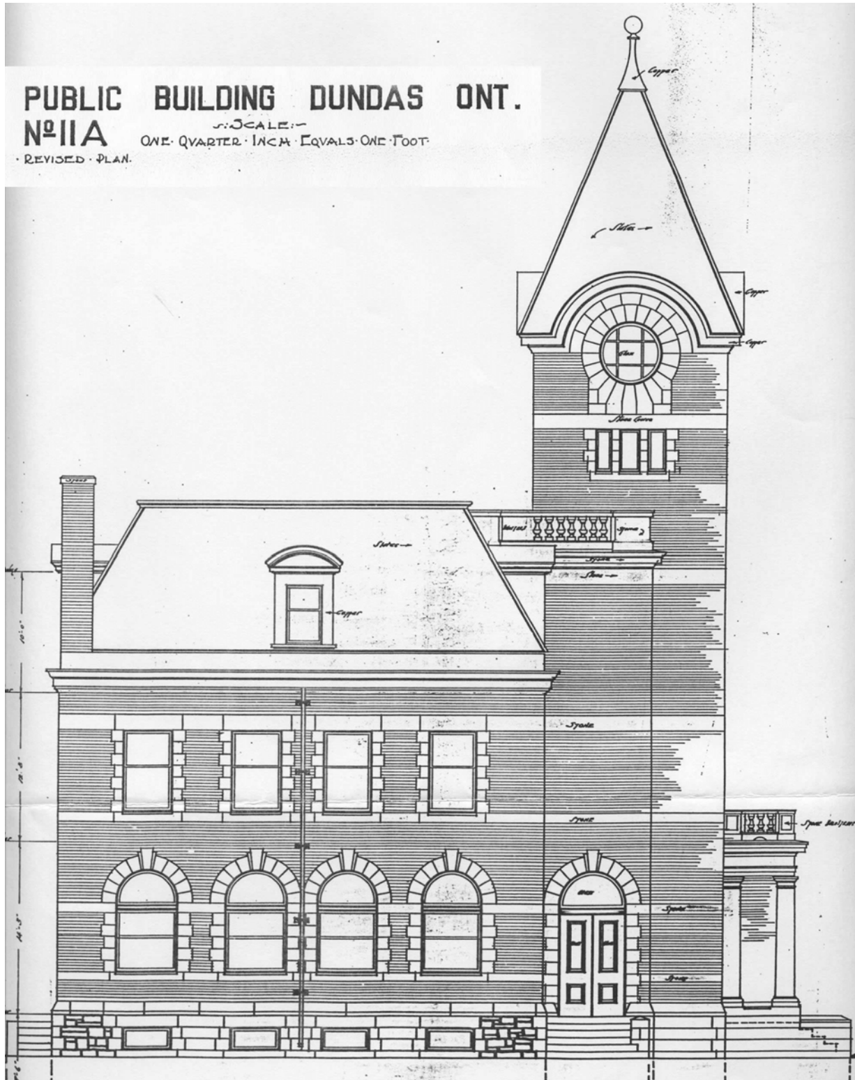
Figure 25: Drawing No. 11A (1911): Foundry Street Elevation (east), showing the original entrance on the east wall of the frontispiece (identical to its west doorway).
