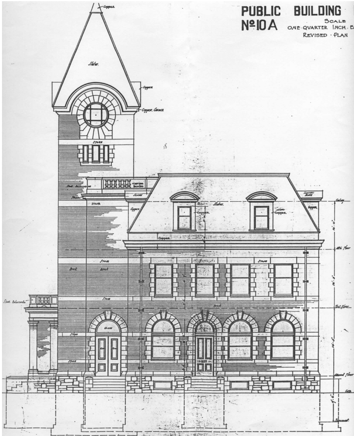
Figure 24: No. 10A (1911): McMurray Street Elevation (west), showing the original entrance of the west side of the frontispiece, with its double wood doors and semi-circular transom, and a similar narrower doorway with a single four-panelled door to the south. As built, this doorway had a three-panelled door with a glazed upper panel, as illustrated in Figure 34 .
