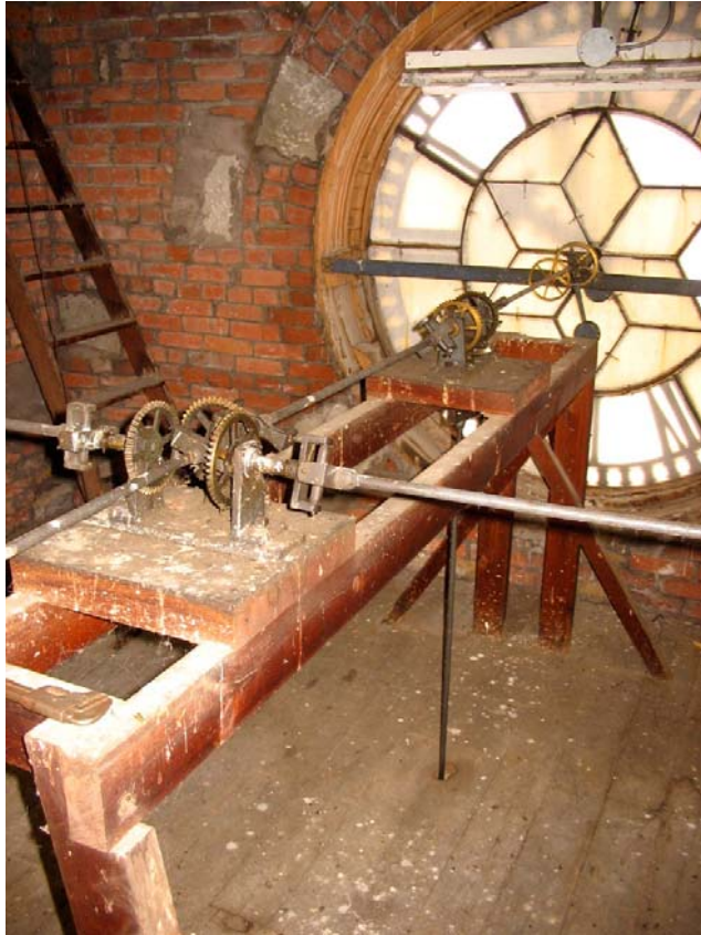
Photo 82 (left): Clock dial assembly showing the vertical drive shaft going through the floor to attach to the mechanism on the fourth floor.
