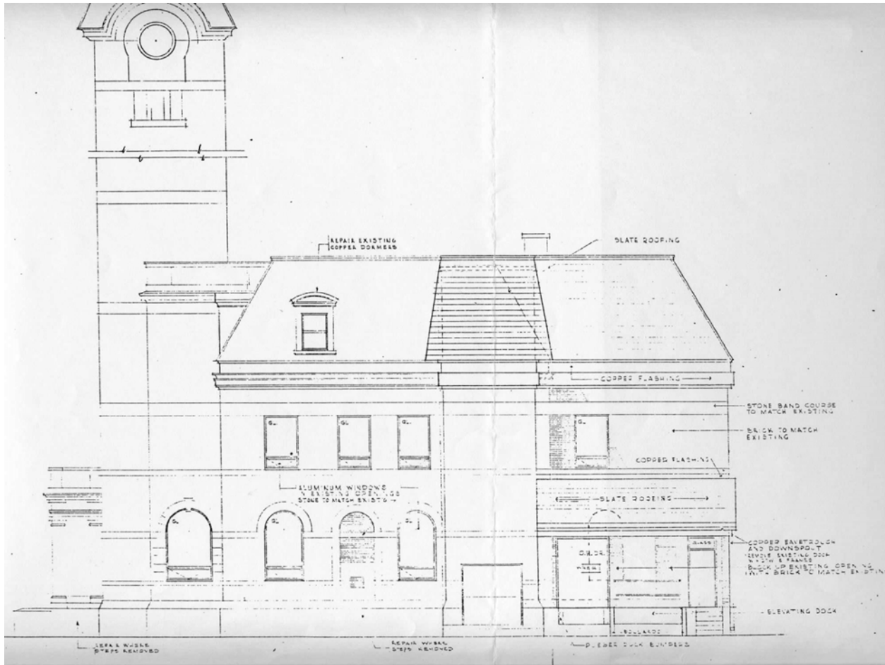
Figure 44: Drawing No. A6: West elevation from the 1978 set of drawings for proposed renovations and additions, showing the new aluminum windows, the second storey addition with a slate mansard roof (also to be wrapped around the mechanical room on top of the elevator shaft), the removal of one of the original round arched windows and half of the double doorway to the Mail Lobby of the pre-1949 rear extension (as shown in Figure 42). Two new doorways were to be installed: an overhead rolling metal door to the left of the new elevating dock and a single doorway with a transom to the right providing access to the new rear stairwell. The concrete platform as reconfigured for these new doorways and elevating dock was to be covered with a shed-roofed addition.
