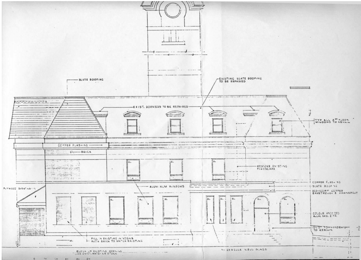
Figure 45: Drawing No. A7: South elevation from the 1978 set of drawings for proposed renovations and additions, showing the new aluminum windows and door (original doorway for the customs receiving room), the shed-roofed porch addition with the masonry end wall over the loading dock on the west facade, and the two ground floor and two basement windows in the pre-1949 extension to be permanently blocked up. A comparison of this elevation with the 1911 one (Figure 20) shows that the original doorway to the west of the arched doorway had already been replaced with a window. Since 1979, the two narrow windows have been located in the women’s washroom and the single wider one in men’s washroom.
