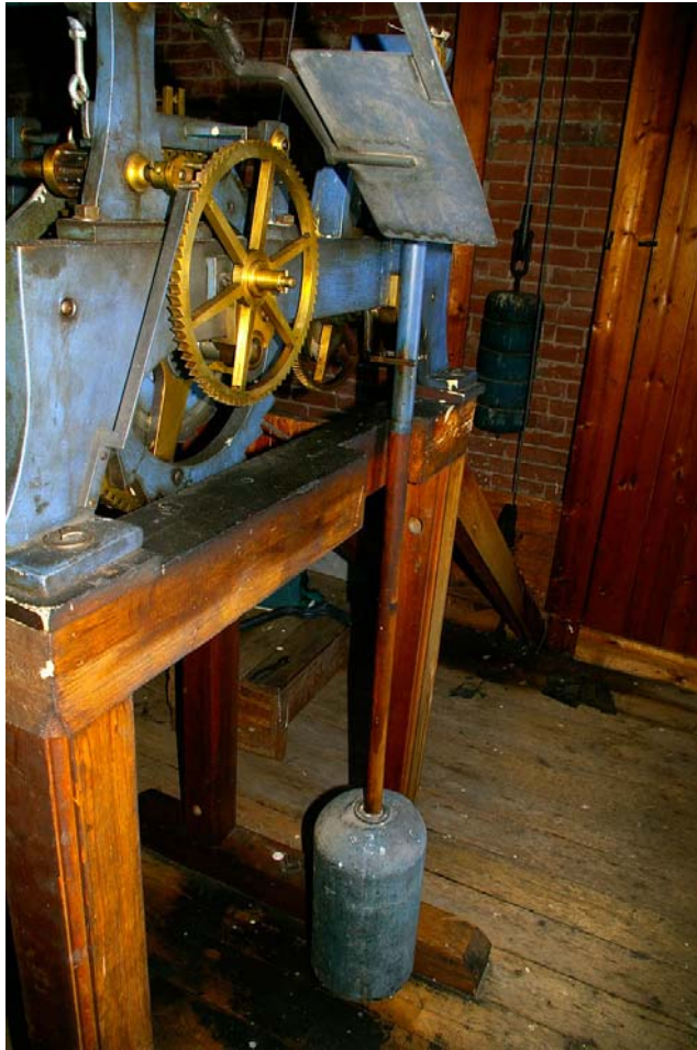
Photo 74: Bell and clock mechanism showing the clock pendulum and the counterweight for the bell hanging in front of the brick wall on the west side of the tower.
