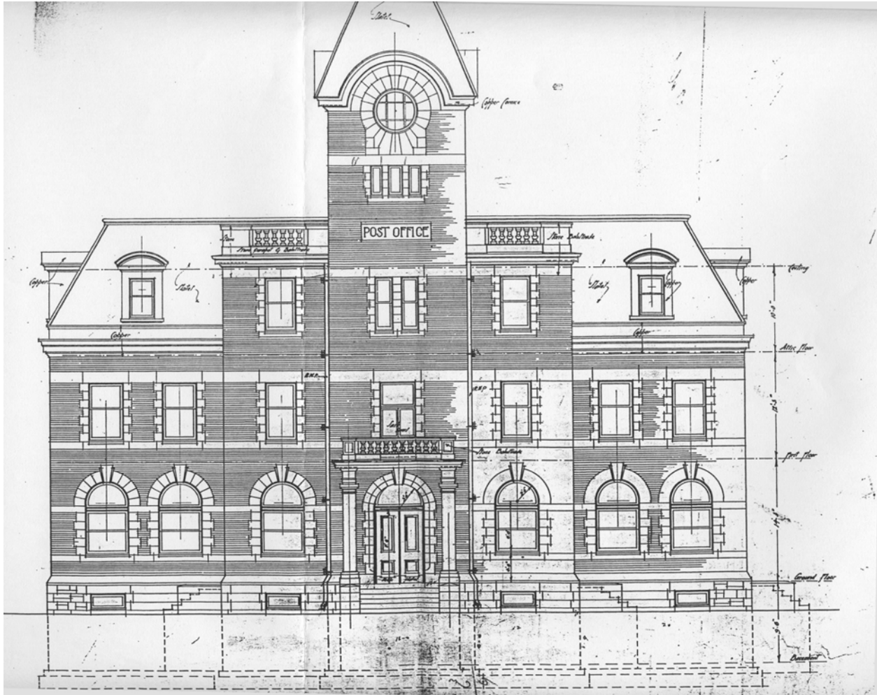
Figure 22: Drawing No. 8A (1911): King Street Elevation (north), showing the original front doorway inside the portico, with its glazed double paneled doors and semi-circular transom. Dotted lines show the below grade foundation walls, footings and basement walls. This elevation and the east and west elevations show the circular openings for the clock dials filled with multi-paned wood windows.
