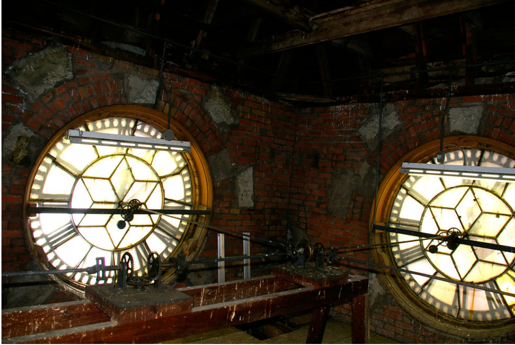
Photo 80: Two of the clock dials and the rods connecting them to the vertical drive shaft which is attached to a gear on the mechanism below.
