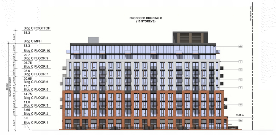
3 SOUTH ELEVATION - BUILDING C SPA305 1:250
