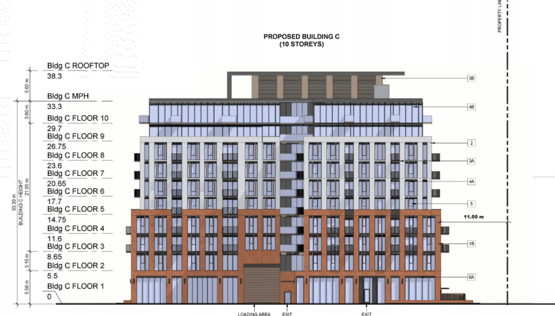
4 WEST ELEVATION - BUILDING C SPA305 1:250
