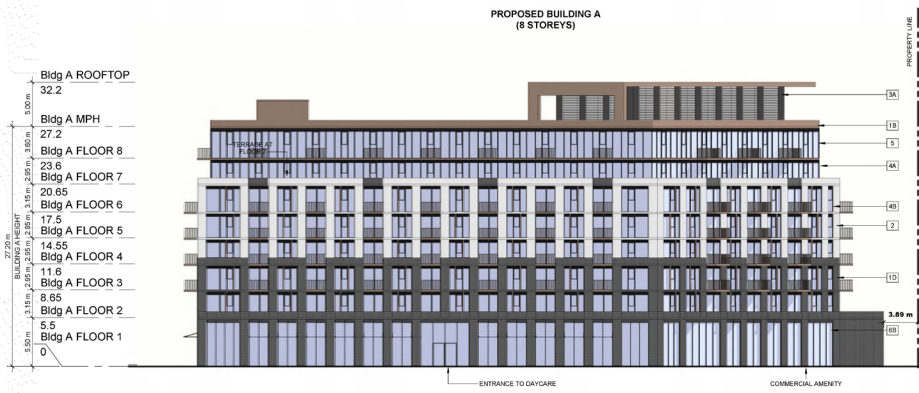
1 NORTH ELEVATION - BUILDING A SPA303 1-200
