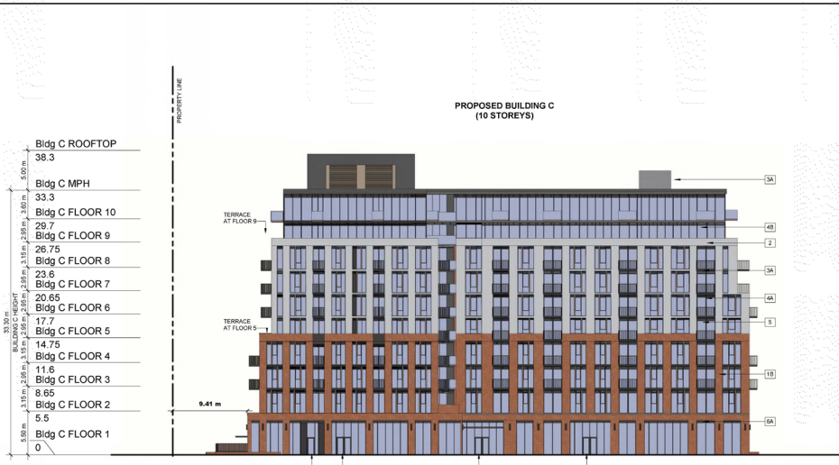
2 NORTH ELEVATION - BUILDING C SPA305 1:250
