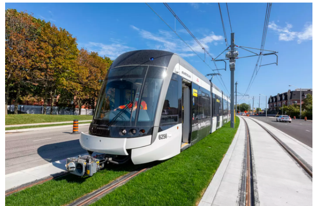
Figure 4.7: Green trackbed in Scarborough
