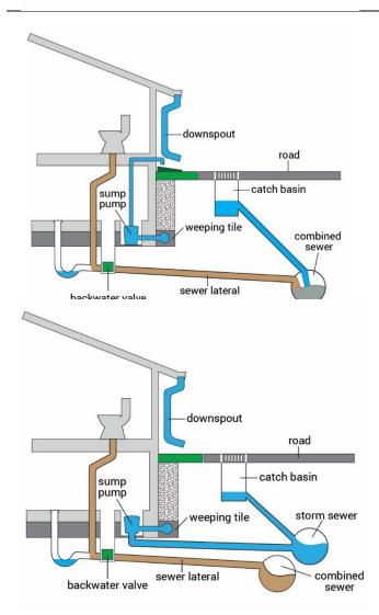
Best Practice recommends that downspouts discharge to the ground surface, and the Foundation Drain should discharge to the ground if the soil conditions permit or connect to the Storm Sewer if available Authority: Item 9, Public Works Committee Report 07-016 (PW07153) CM: December 12, 2007 Ward: 2, 7
