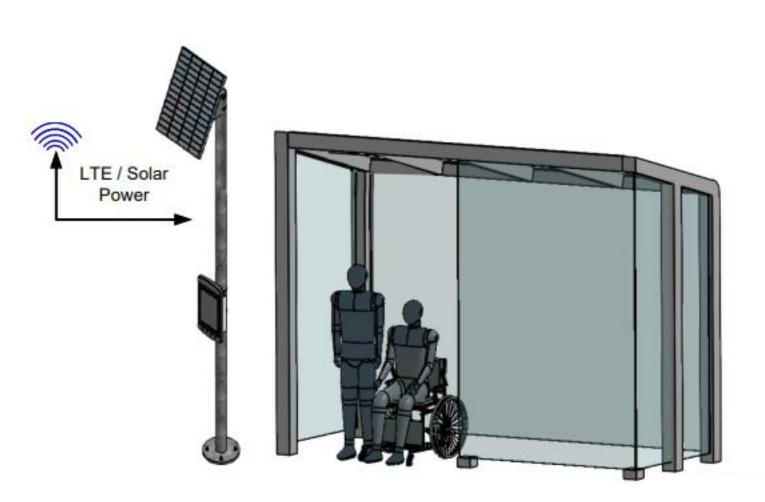
Digital illustration of how a display unit may look at a bus stop, with the display pole on the left and the bus shelter on the right, depicting two customers waiting.
