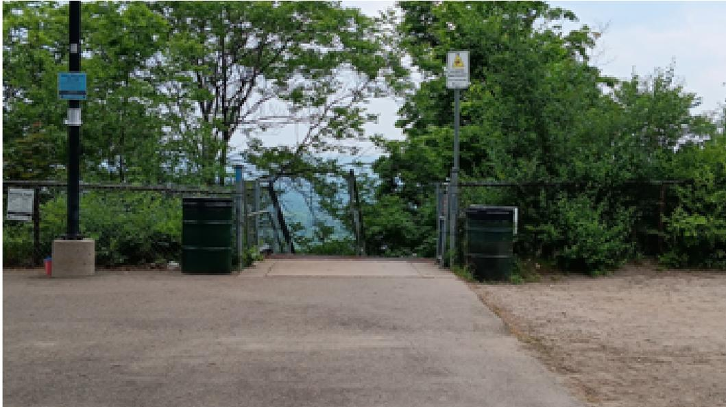
The approach to the upper entrance to the stairs has good sight lines. There is some vegetation growing through the chain-link fence. This can be pruned back. The garbage cans should be relocated further from the stairs. This will eliminate a potential concealment area.
