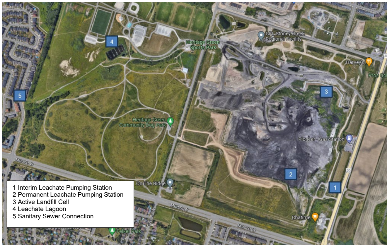
Figure 2.1 Leachate Collection and Disposal Network
