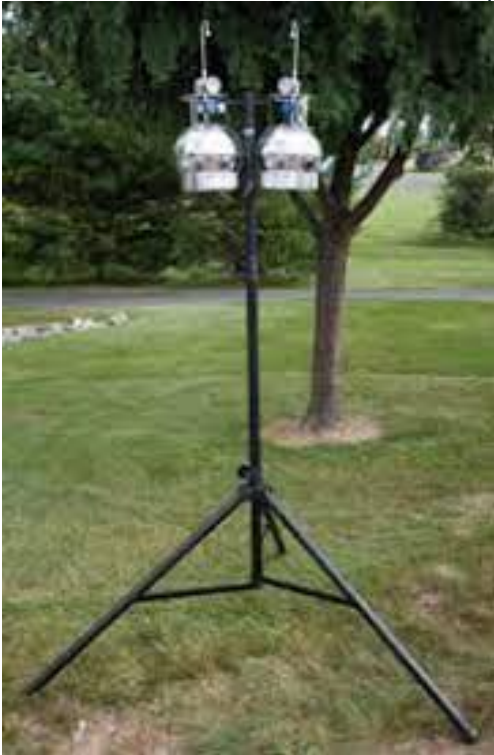
Short-Term Fixed Location Canister Sampling Equipment
