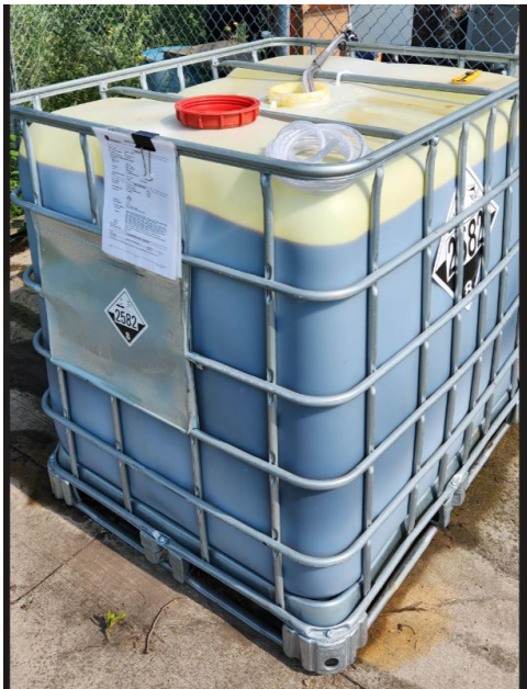
Figure 2 Ferric Chloride Tote
