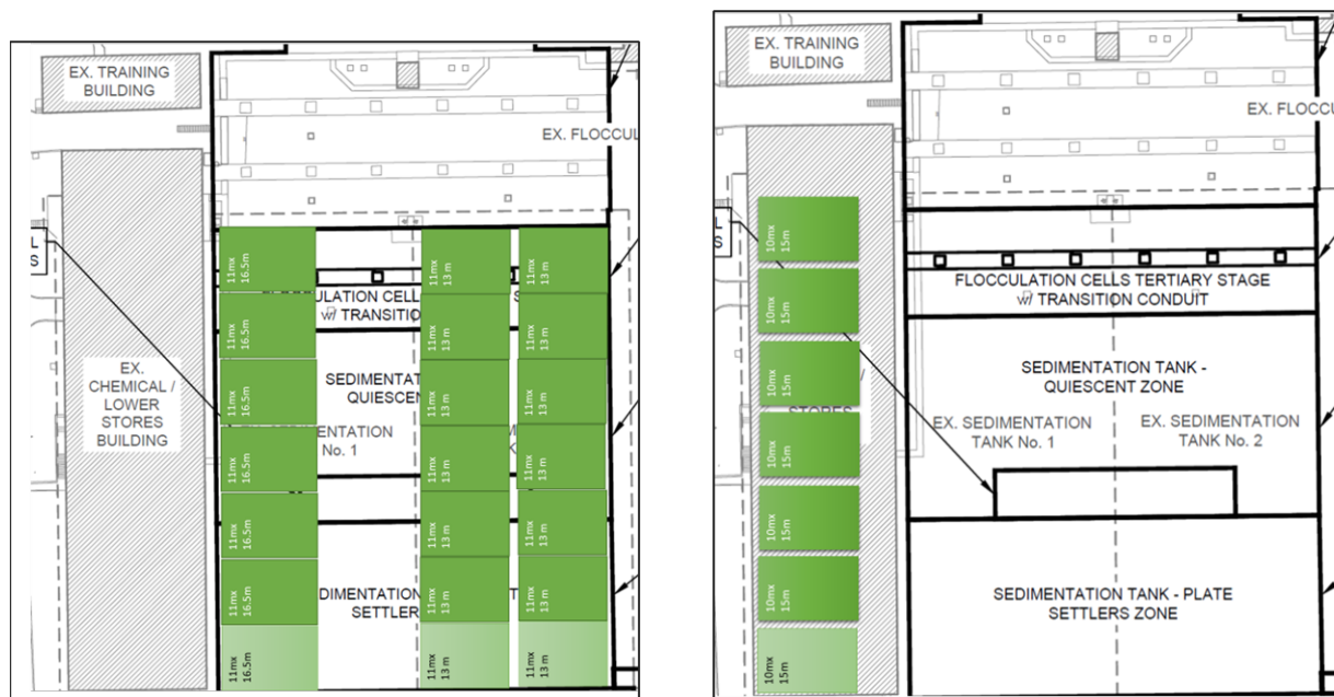
Figure C-2: Preliminary conceptual schematic of DAF unit process layouts; retrofit into existing sedimentation basins (LEFT) and greenfield construction in location of existing lower stores (RIGHT).
