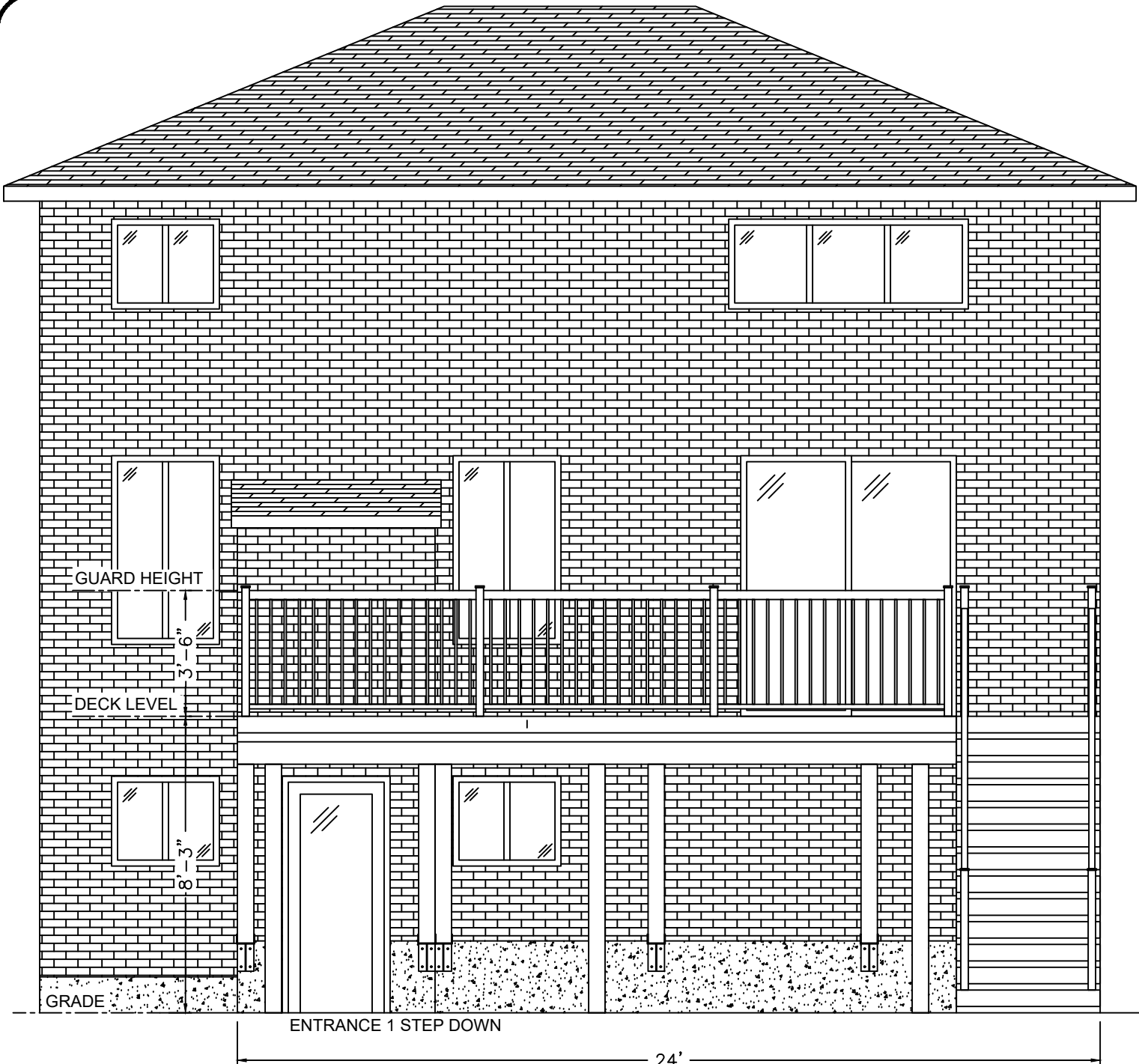
1 DECK FRONT ELEVATION SCALE: 1/4" = 1' - 0"
