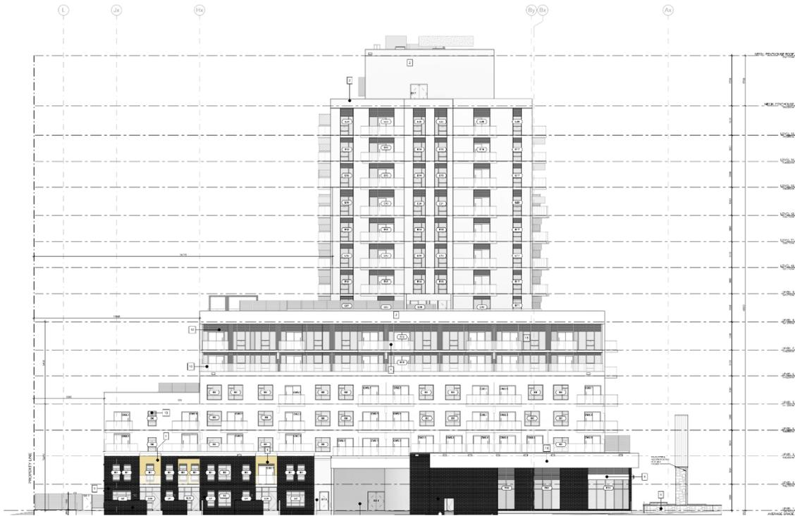
Figure 6: Eastern Building Elevation (Source: SRM Architects)
