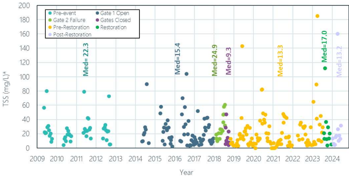
Figure 4.7: Chedoke Creek at CC-SW2/CP-11 TSS Concentrations (2009 through 2024)
