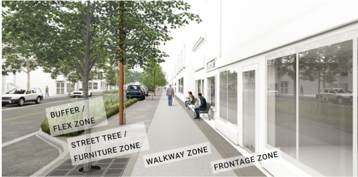
Figure 1 - Illustration of pedestrian zones. Source: City of Hamilton Complete Streets Design Manual
