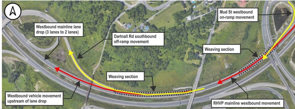
Figure 23: Existing Design Issues - Dartnall Road Interchange
