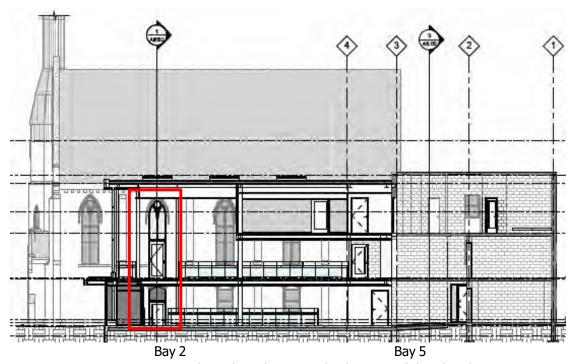
PROPOSED ADDITION Section through to the east side elevation of the Church – existing windows in Bay 2 will be modified for doorways into the new addition – the upper portions of these windows will remain
