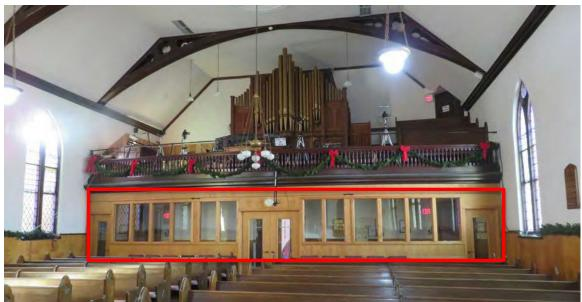
Proposed Interior Alterations to the Sanctuary - partition wall installed in 1991 to be removed - Gallery to remain
