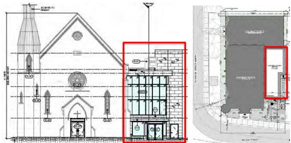
Proposed Addition on the east side of the Church – glazed front wall and new landscaping on Wilson Street – interior space in the addition is organized around an atrium to minimize impacts on the east wall of the Church – skylights in the roof will provide natural light to illuminate the stained glass windows in the atrium
