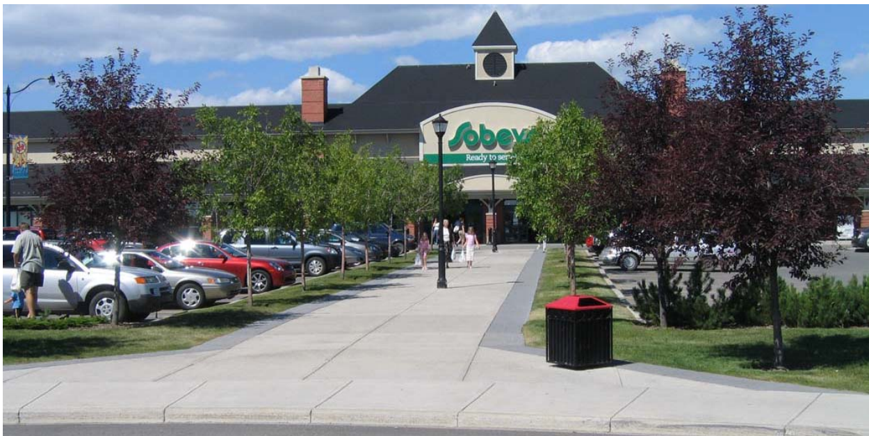
Photo 5.19: A network of pedestrian crossings should be incorporated on large commercial sites, including sidewalks located in the front of buildings.
