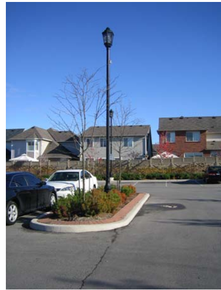
Photo 5.29: Smaller "parking courts" should be created using raised and curbed traffic islands planted with trees and low level vegetation to maintain visibility.
