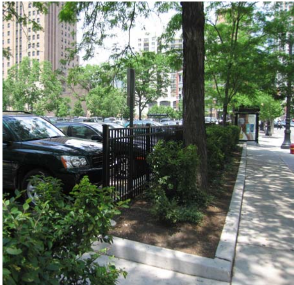
Photo 5.30: Adequate buffers should be provided between parking areas and public sidewalks.
