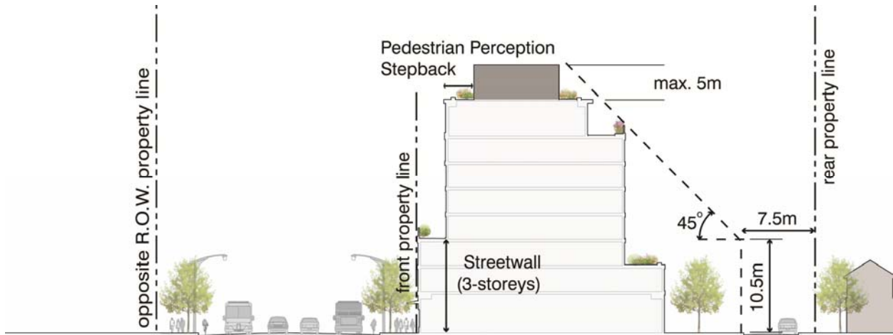
Figure 5.1: Angular planes and setbacks are recommended to define a building envelop in the Mixed Use Medium Areas that creates a comfortable pedestrian realm, and ensures appropriate transitions to adjacent uses.
