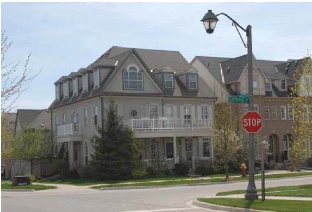
Photo 4.3: Both lot frontages on corner lots should have positive expression to the street through front porches and projecting bays, windows, etc.
