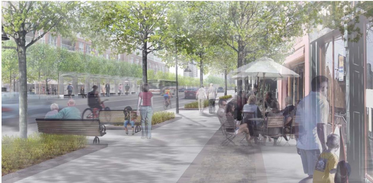
Figure 3.6: Retail and Mixed Uses intended to front onto Collector Road A should have a pedestrian scaled (2 to 4-storey) building base with large amounts of clear glazing, and opportunities to sit and socialize.
