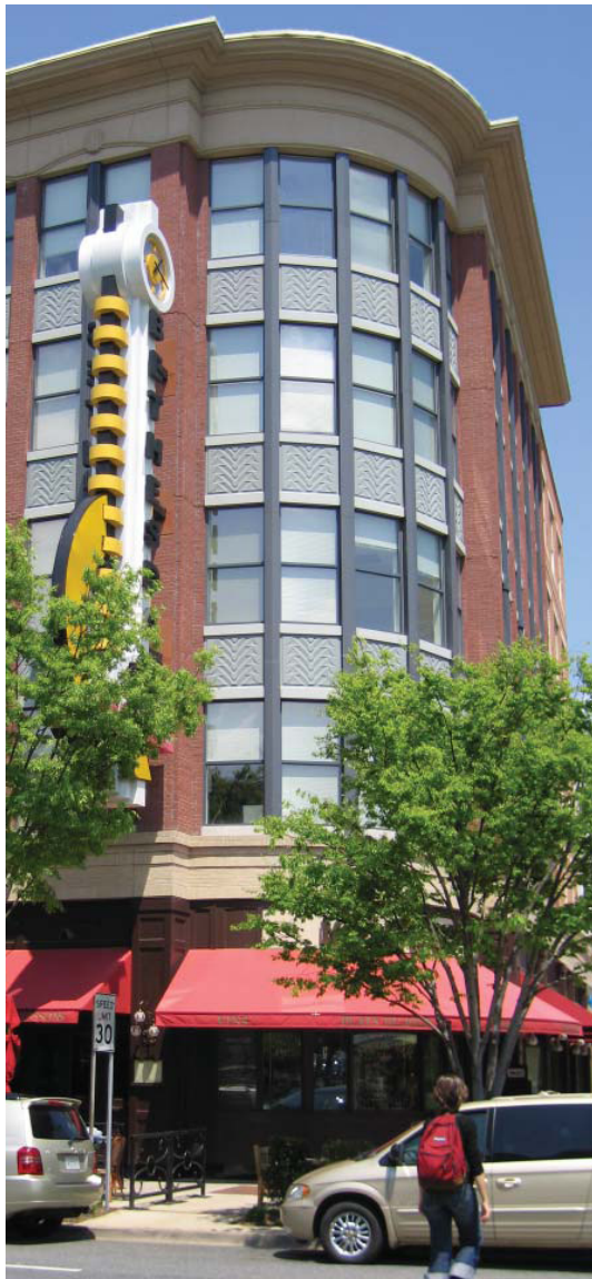
The massing of buildings at important focal points such as the corners of major intersections should be configured to reflect their important location
