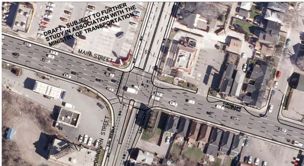
Exhibit 6-24: Option 1- Left Turn Lane on Main Street West at Dundurn Street (MTO Issue)
