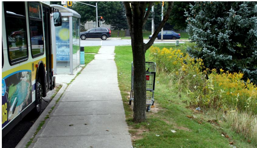
A non-accessible stop which lacks a physical barrier between the deployment area and a steep slope
