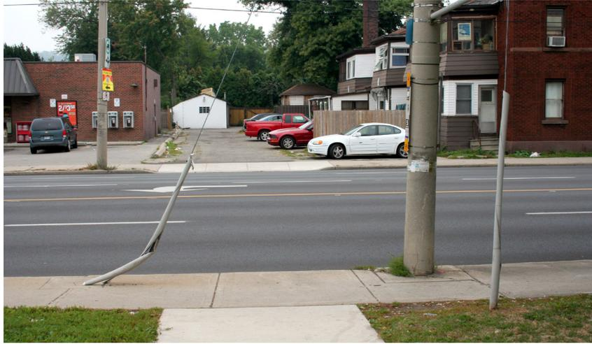
A non-accessible bus stop with a utility guy wire obstructing the landing pad area, without any reflective sheath
