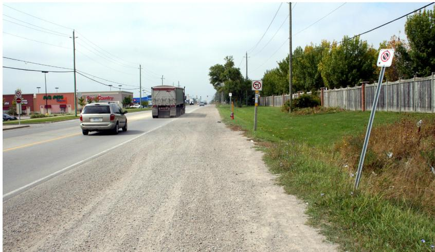
Non-accessible bus stop on a rural road with no landing pad or sidewalk
