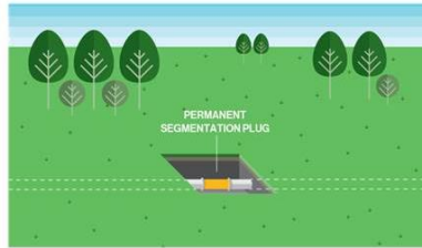
4. Segment the pipeline with permanent physical barriers to prevent it from acting as a water conduit. Segmentation plugs are strategically placed along the pipeline.
