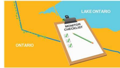
5. Monitor the pipeline, by maintaining cathodic protection, regular patrols, exact location signs, depth-of-cover surveys and Click Before You Dig program information.
