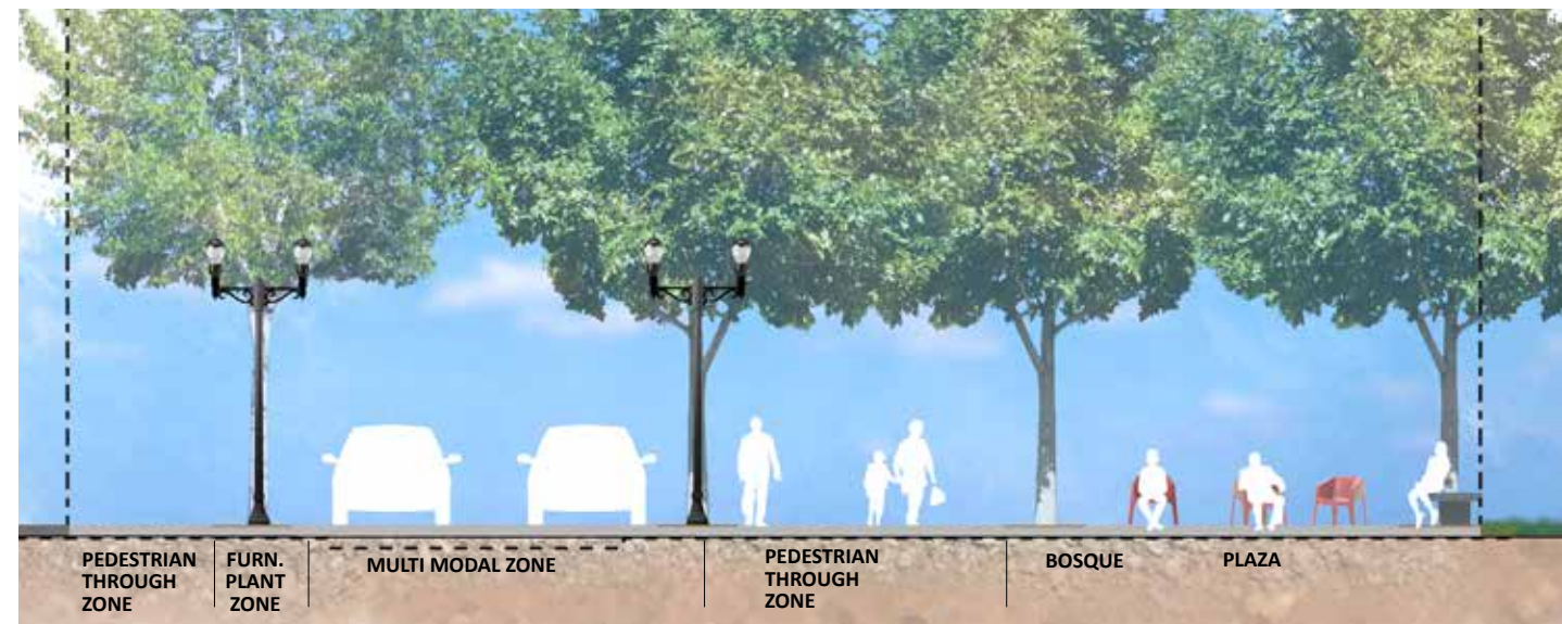
FIGURE 2.4.2: A - A' CONCEPTUAL HUGHSON STREET CROSS SECTION: LOOKING NORTH
