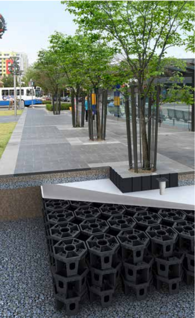
FIGURE 3.3.3.5: STRUCTURAL SOIL CELLS PROVIDING INCREASED SOIL VOLUMES FOR TREE GROWTH. ILLUSTRATION: CITY GREEN.
