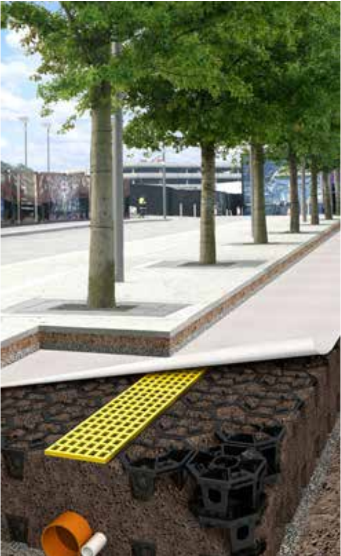
FIGURE 3.3.3.6: STRUCTURAL SOIL CELLS IN A CONTINUOUS TRENCH.
