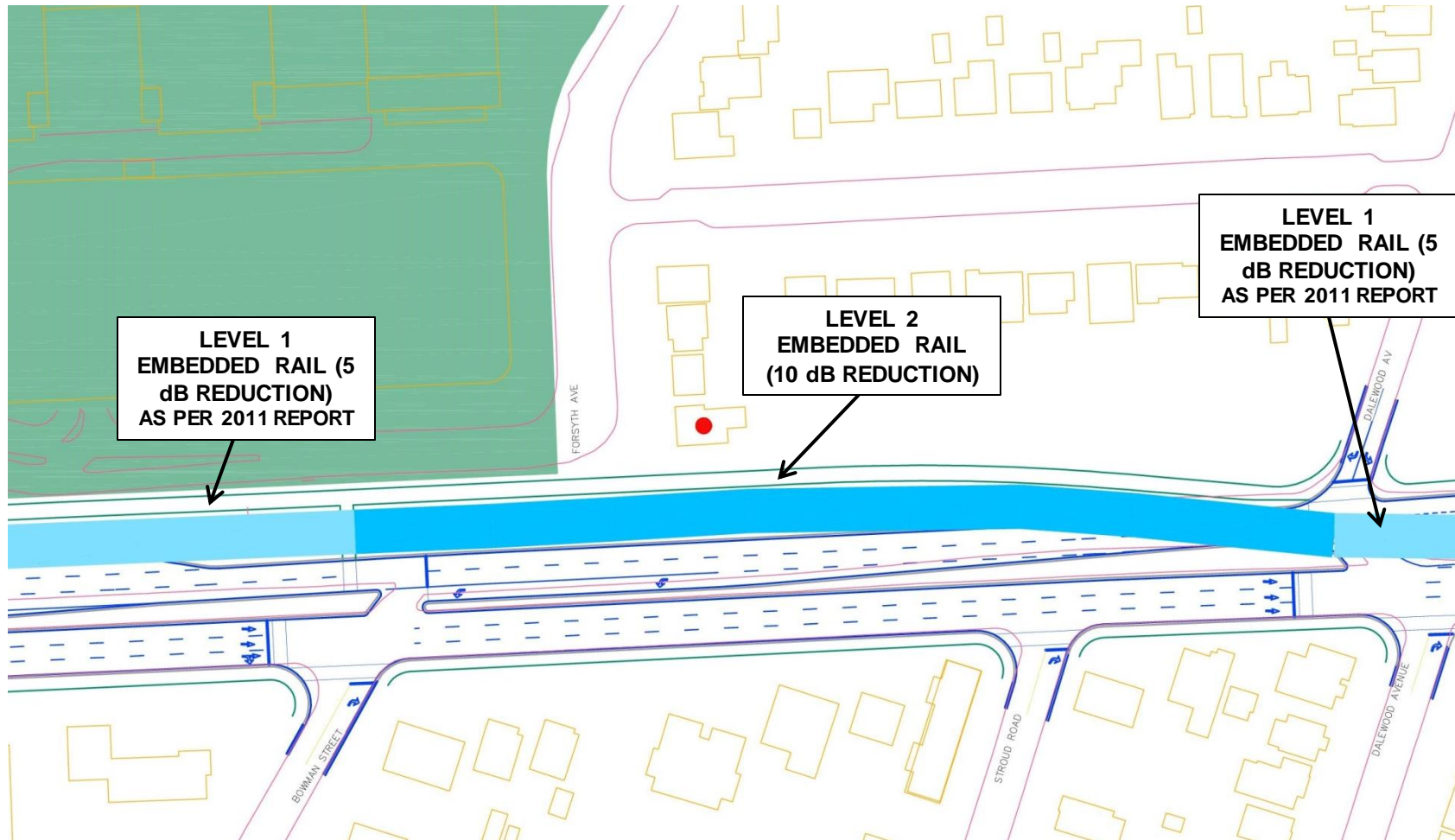
Figure 9: Vibration Control Recommended for Receptor 11
