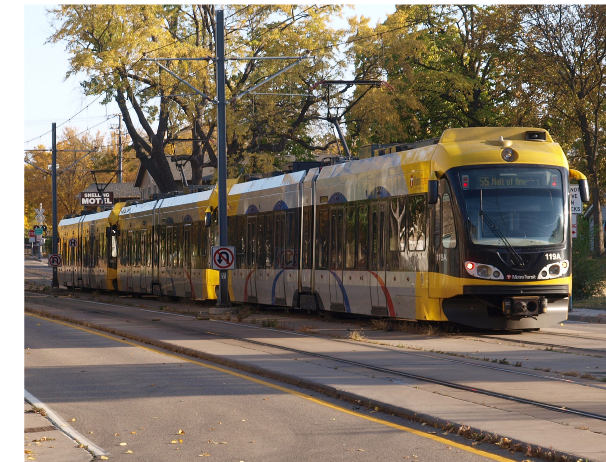
↑ Centre-pole catenary system in Minneapolis (centre-running with one traffic lanes on each side)
