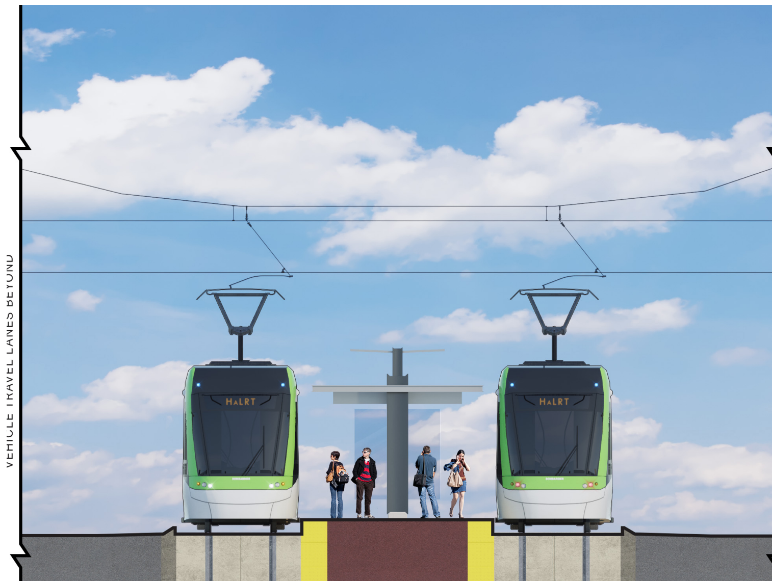
Typical centre stop platform
