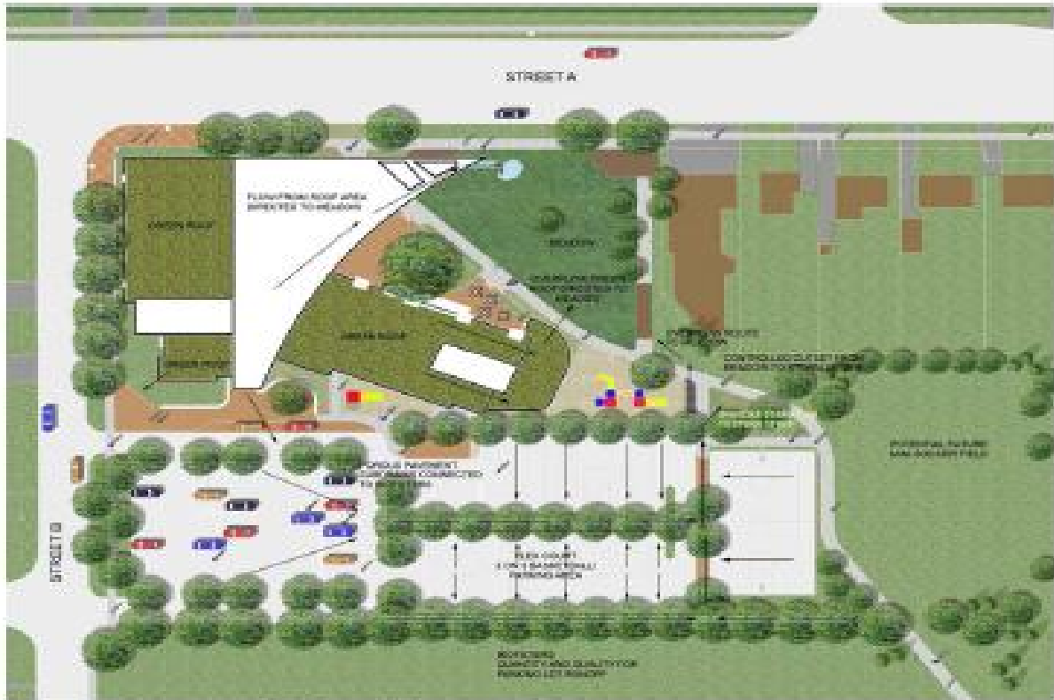
Figure 6.3: Example Landscape-Based LID Stormwater Management Strategy
